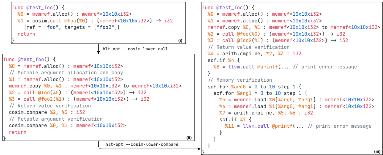
Figure 4.7: Lowering of cosim dialect operations. A cosim.call operation (i) is lowered into two function calls (ii), mutable argument copying and side-effect comparison (iii) using cosim.compare operations. cosim.compare operations are lowered into verification code in (iii), which can be further lowered to executable LLVM IR.
