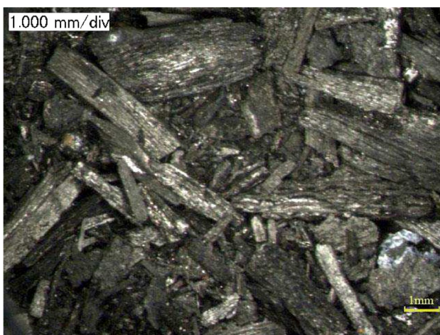
Fig. 2 Microscopic (25 times enlarged) view of wooden charcoal
