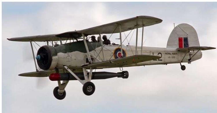
Figura 46. Fairey Swordfish com torpedo de 18” (45 Cm) e 1610 lb (730 Kg).
