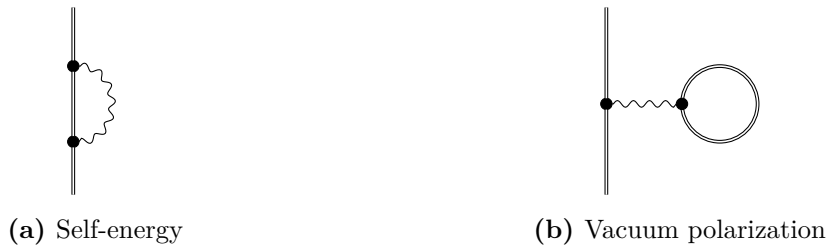
Figure 2.2: Feynman Diagrams for the main radiative quantum electrodynamics correction performed on atomic structure calculations.
