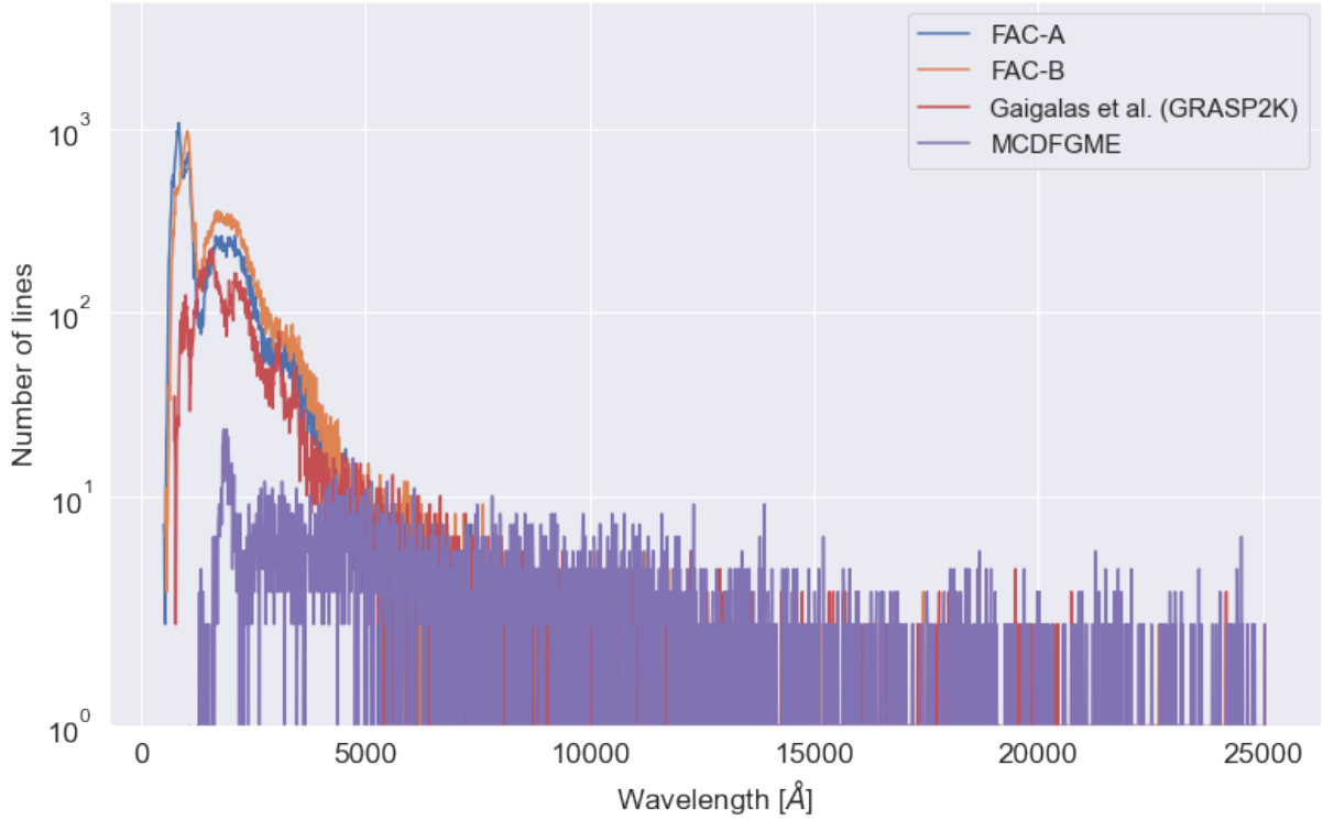
Figure 3.8: Number of strong transitions for Nd III as a function of the wavelength obtained with both FAC calculations and with the MCDFGME calculations compared with the results of GRASP2K of Gaigalas et al.
