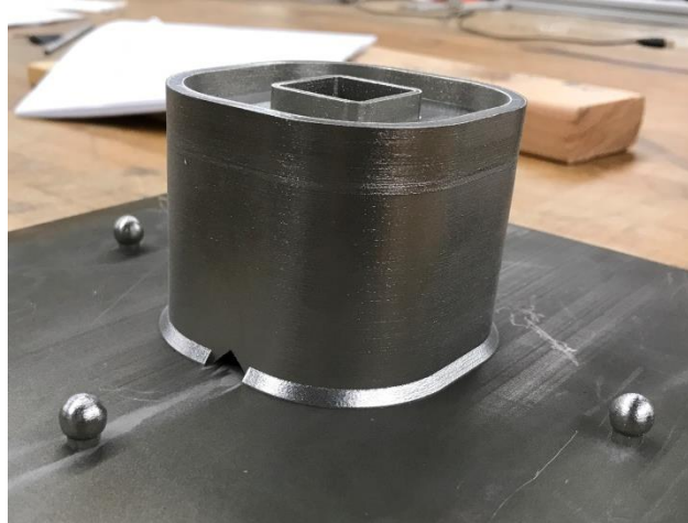
Figure 2.10: Square Canonical Structure Built by the EOS M290 DMLM Process
