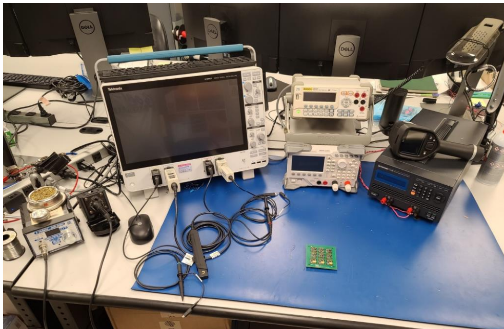
Figure 8: Test equipment used for testing various PoL converters
