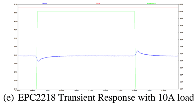
Figure 10: EPC2218 simulated waveforms at 3.3V
