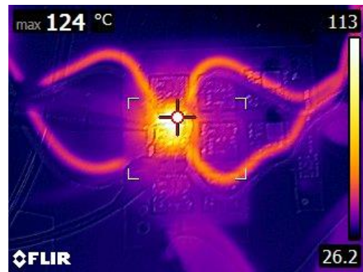
(d) Loaded steady-state operation of the EPC2030 at 2 MHz for 3.3V output
