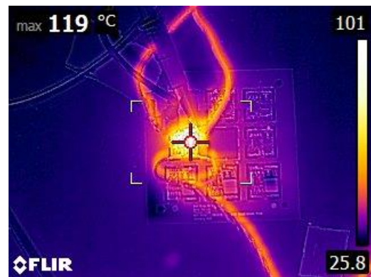
(f) Loaded steady-state operation of the EPC2218 at 2 MHz for 3.3V output
