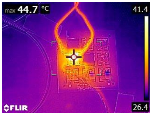
(e) No-load steady-state operation of the EPC2218 at 2 MHz for 3.3V output
