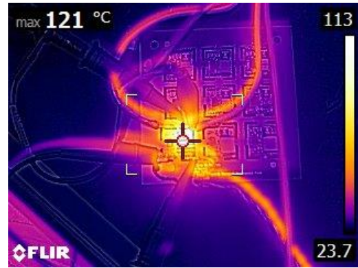
(b) Loaded steady-state operation of the GS61008T at 2 MHz for 3.3V output
