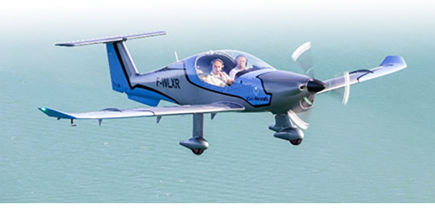
Fig. 1. The Elixir, EASA certified two-seater light aircraft ( https://elixir-aircraft.com ).
