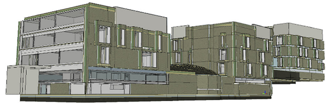
Fig. 1. 3D climate, comfort, and energy simulation model of the Szentágothai Research Center reference building (software: IDA ICE 4.8)
