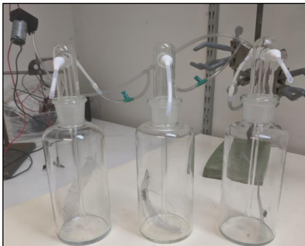
Figure 4. Glass bottles for headspace sampling of volatile compounds. Pheromones produced by beetles were pumped into collectors adsorbing the compounds. The picture displays a male and female timberman beetle ( Acanthocinus aedilis ) subjected to headspace sampling. (photo: B. Eriksson)
