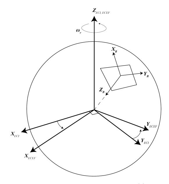
Figure 4.1: Coordination systems related to attitude on satellites. {B} is the body frame, {ECI} is the Earth-centered inertial frame located at the center of Earth and fixed, {ECEF} is the Earth-centered, Earth-fixed frame situated in the center of Earth and rotates.
