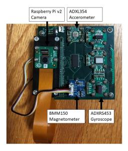
Figure 4.7: Sensor suite testing board
