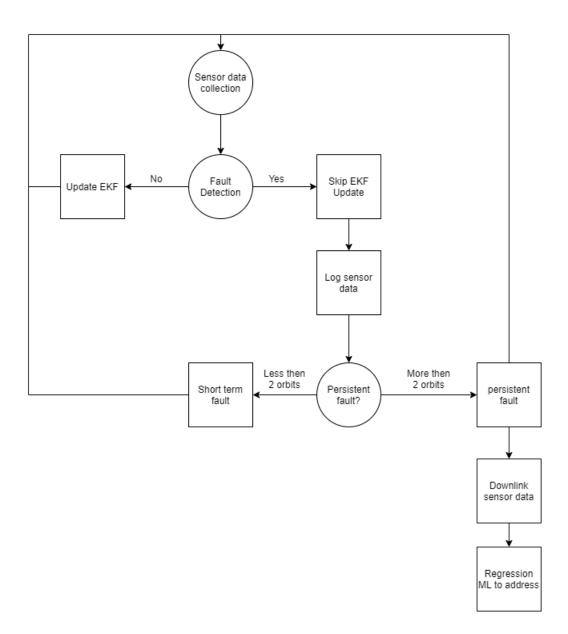
Figure 4.12: Fault detection process flow diagram
