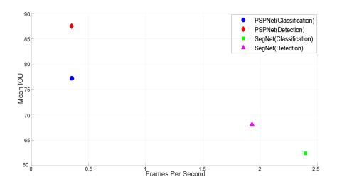
Figure 3.8: Speed vs. mean IOU for both architectures for both datasets. A clear divide between accuracy and speed is presented between both models. The running time is measured on an AMD Ryzen 7 3800X with 32 GB of RAM.
