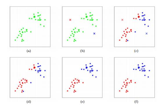
Figure 2.1: Example of how k-means clustering works, the dots represent the training examples, and centroids are represented by the crosses. (a) the original dataset.(b) random initialization of the clusters. (c-f) the k-means clustering algorithm is demonstrated as the points are reassigned and new centroids are defined [2].
