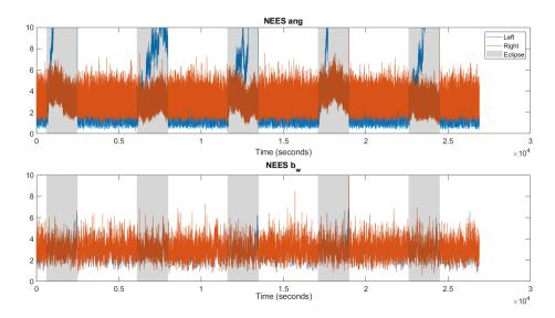
Figure 4.6: The left and right quaternion error parameterization NEES performance for five full orbits simulation.
