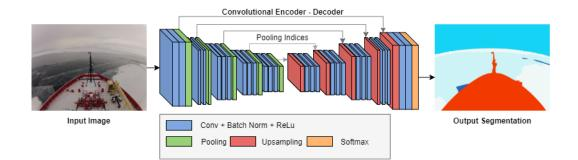
Figure 2.3: The structure of the SegNet encoder-decoder architecture [4].
