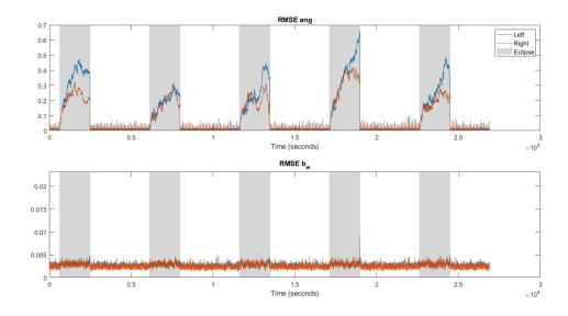
Figure 4.5: The left and right quaternion error parameterization RMSE performance for five full orbits simulation.
