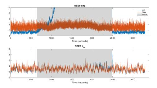
Figure 4.4: The left and right quaternion error parameterization NEES performance for one full orbit simulation.
