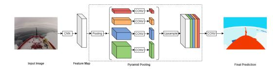
Figure 2.4: The architecture of the PSPNet model, in the case of the PSPNet101 model implemented, the CNN input seen in the figure is the ResNet101 model [5].
