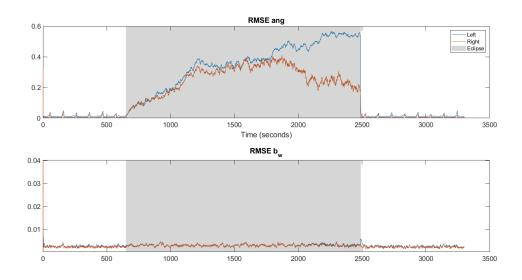
Figure 4.3: The left and right quaternion error parameterization RMSE performance for one full orbit simulation.
