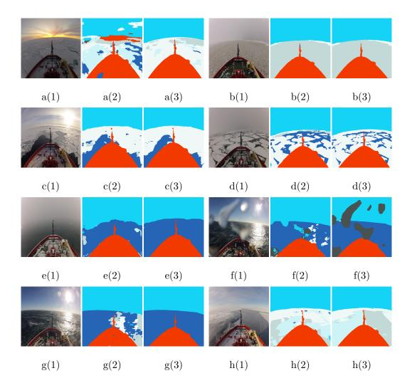
Figure 3.6: Comparison of segmentation results of both ice classification models using test images. (1), (2), (3) are used to indicate the image, SegNet prediction of classes, and PSPnet prediction of classes, respectively, with the boat in red, the ocean in dark blue, the sky in cyan, first-year ice in white, grey ice in grey-blue, and new ice in pale blue. In images, both neural networks' overall segmentation performances are observed on images from the test set.
