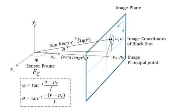
Figure 4.8: The sun sensor calculation technique
