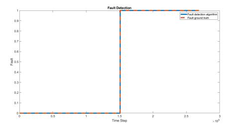
Figure 4.15: The results of the fault gating with a magnetometer bias increase half way through the third orbit.
