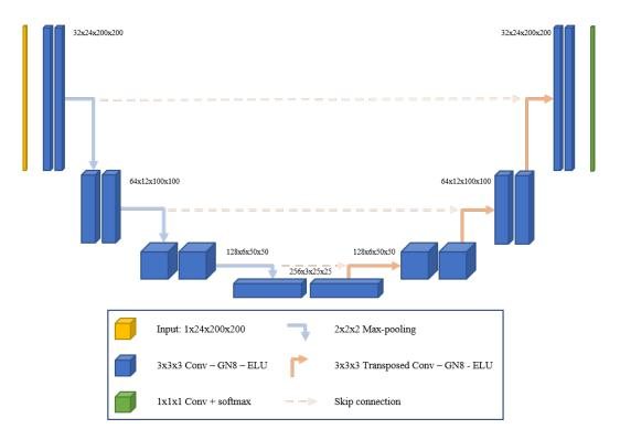
Figure 2.2: The U-net architecture. Each blue box corresponds to a multi-channel feature map. The arrows denote the type of operation. The dashed lines represent the skip connection between each corresponding encoder decoder layer [3].
