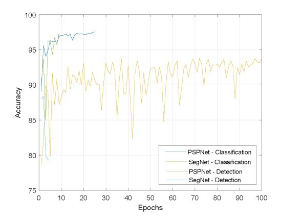
Figure 3.4: pixel-wise accuracy for the validation sets of both neural networks for the ice classification dataset and the ice detection dataset
