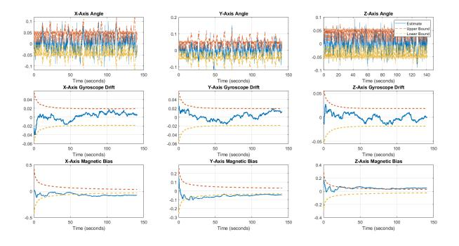
Figure 4.16: The results of the sliding window batch optimization to detect the unknown magnetic bias. The first row represents the Euler angle estimation, the second row is the gyroscope drift, and the last row represents the magnetic bias estimate.
