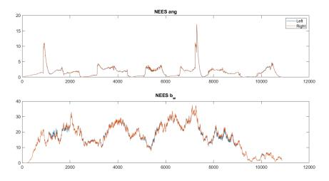
Figure 4.11: The left and right quaternion parameterization NEES performance for the nine minute lab physical testing.
