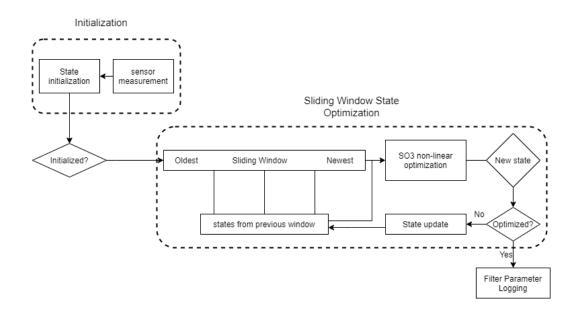
Figure 4.13: A flow diagram of the sliding window filter using regression machine learning to estimate the magnetic bias state.
