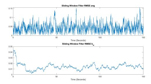
Figure 4.17: The RMSE results of the sliding window batch optimization for a small period of the simulation.
