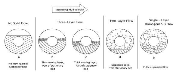
Figure 4-12: Transition of a stationary solid bed to fully suspended flow.
