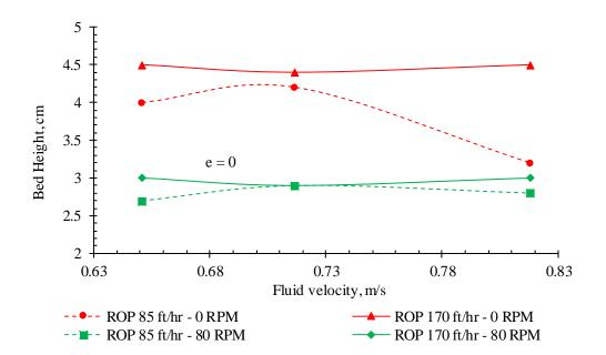
**Figure 3-16**: Effect of rate of penetration (ROP) on bed height (e = 0)
