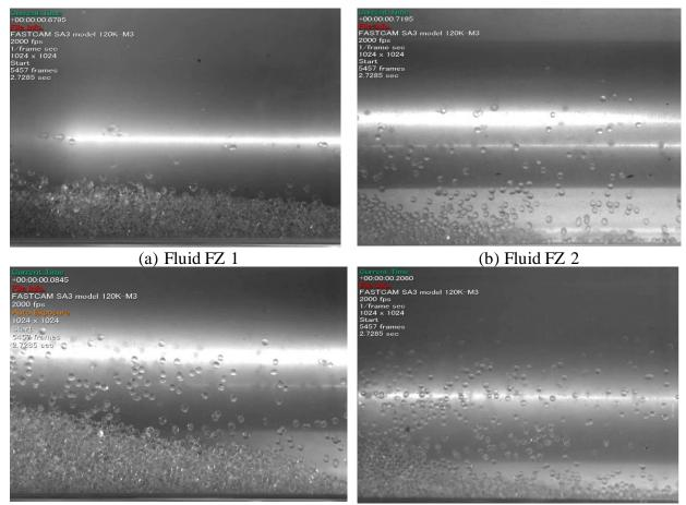
(c) Fluid FZ 3 (d) Fluid FZ 4 **Figure 4-10**: Visualization of the high-speed camera for different fluid rheology. Increasing the fluid viscosity shows a higher solid content in a suspended form in the mud  $(\mu_{FZ1} < \mu_{FZ2} < \mu_{FZ3} < \mu_{FZ4}).$
