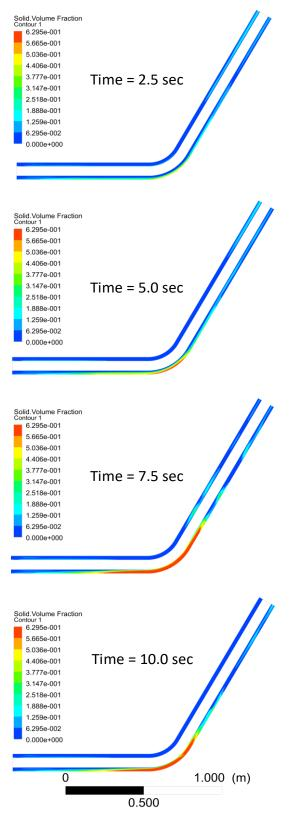
Figure A.5: Solid cuttings accumulation in the bend section with time.
