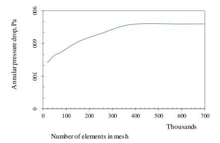
Figure A.3: Grid independence study to choose optimum element in meshing.
