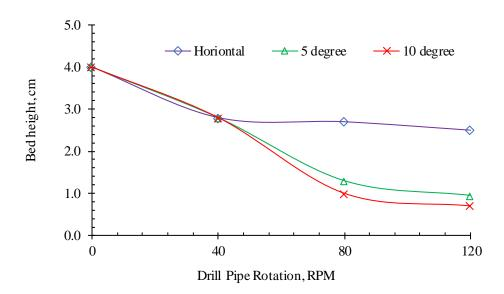
Figure 5-20: Solid bed height at different inclination angles with fluid LV
