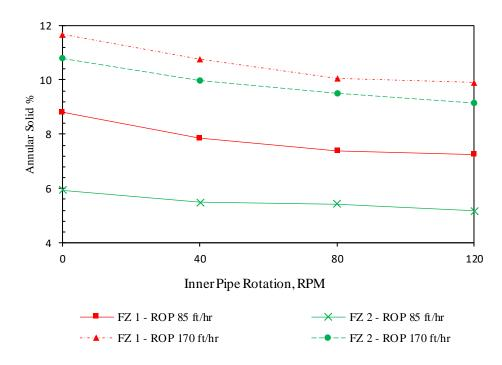
Figure B.7: Annular solid percentage as a function of drill pipe rotation.
