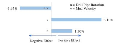
Figure 2-11: The main effects and interaction of field parameters on CTE.
