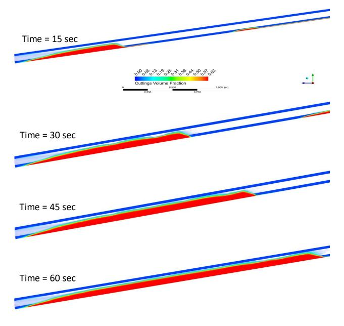
Figure 6-14: Solid dune profile at different time interval
