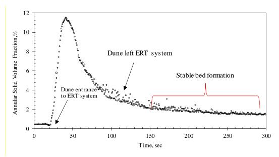
Figure B.5: ERT system shows stable solid bed profile in horizontal well.
