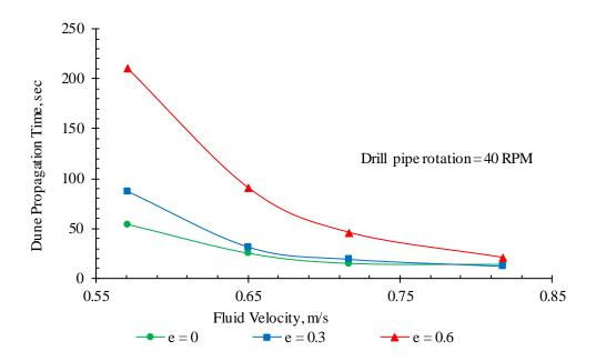
Figure 3-12: Sand dune propagation time for drill pipe rotation of 40 rpm
