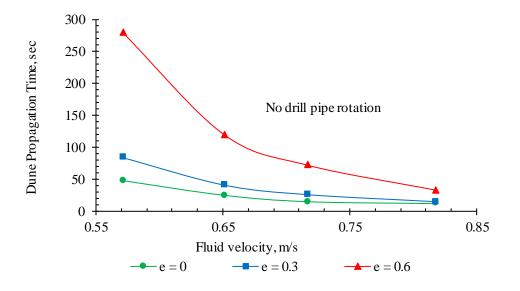
Figure 3-11: Sand dune propagation time for stationary inner pipe (RPM = 0) Figure 3-12 and Figure 3-13 shows dune propagation time for inner pipe rotation of 40 and 80 RPM respectively. Comparing Figure 3-11 with Figure 3-12 and Figure 3-13 shows that, imposing inner pipe rotation significantly reduce the dune propagation time for all cases. For
