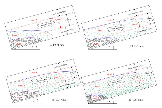
Figure 5-14: Schematic of solid transport in inclined well with change in mud velocity.
