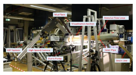
Figure 3-1: Flow loop experimental set up located at TAMUQ, Qatar.
