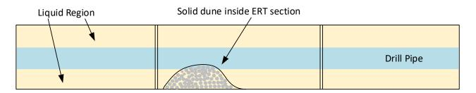
Case 2: Both solid dune and liquid inside the ERT section.
