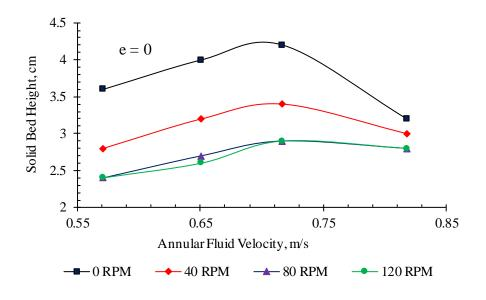
**Figure 3-4**: Effect of annular fluid velocity on solid bed height (e = 0)
