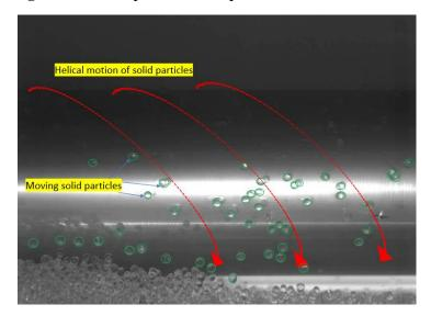
Figure 3-21: Visualization of helical motion of solid particles due to inner pipe rotation.
