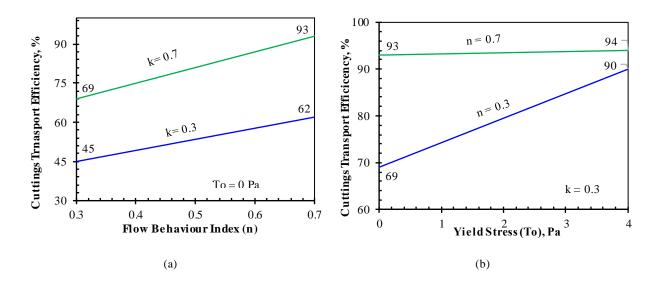
Figure 2-9: Effect of two-factor interaction of a) k and n; b) n and to on CTE
