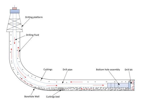
Figure 4-1: Schematic of cuttings transport in horizontal well
