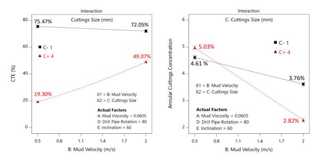
(a) Velocity and cuttings size (BC) interaction effect ontransport efficiency(b) Velocity and cuttings size (BC) interaction effect on
