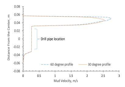
Figure A.9: Mud velocity profile in the horizontal section for 30° and 60° bend.
