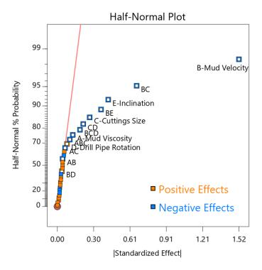
Figure 6-31: Half normal plot for annular cuttings concentration.
