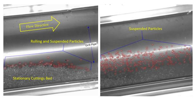
(a) Fluid FZ 1 (b) Fluid FZ 3 **Figure 6-10**: High-speed image (2000 fps) visualization of solid particle movement [10°-inclined well configuration with fluid FZ 1 and FZ 3]
