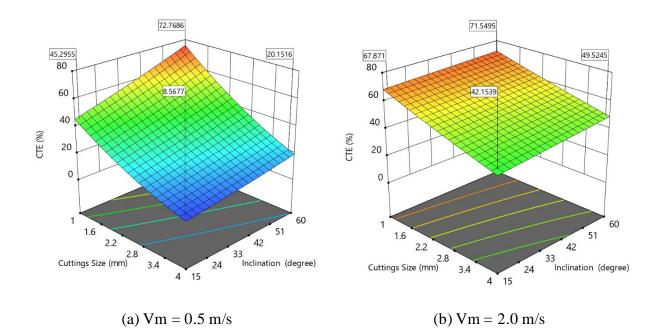
Figure 6-19: Effect of fluid velocity on cutting transport efficiency.
