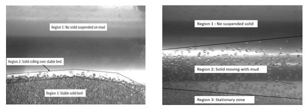
(a)  $V_m = 0.397 \text{ m/s}$  (b)  $V_m = 0.65 \text{ m/s}$
