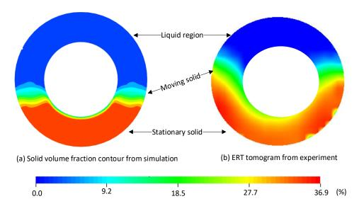
Figure 6-12: CFD Simulation contour vs. ERT Tomogram
