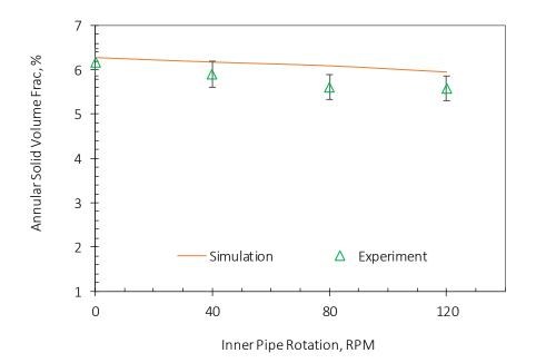
Figure A.4: Experimental validation of CFD model.
