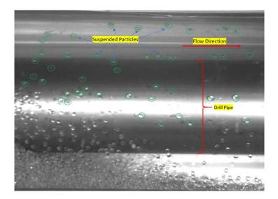
Figure 3-20: Suspended solid particles in the annulus.
