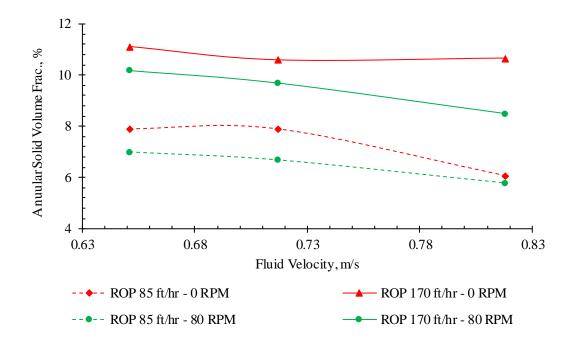
**Figure 3-17**: Effect of rate of penetration (ROP) on annular solid vol fraction (e = 0)
