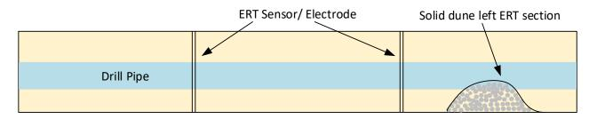
Case 3: Solid dune left ERT section and only liquid inside the ERT section.
