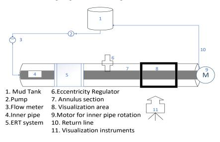
Figure 3-2: Schematic of flow loop experimental set up
