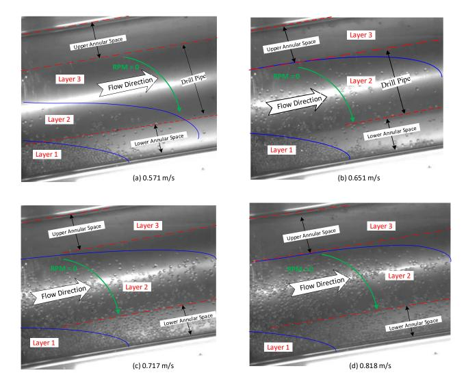
Figure 5-13: Effect of fluid velocity on cuttings transport in 10° inclined well.
