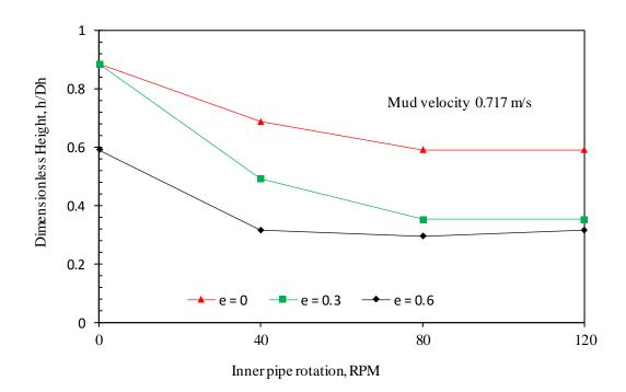
Figure B.6: Variation of bed height with inner pipe rotation for fluid FZ 1. An eccentric annular section (e = 0.3, 0.6) shows a less bed height, compared to a concentric annular section (e = 0).
