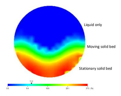
Figure 5-10: ERT concentration tomogram of solid and liquid phases
