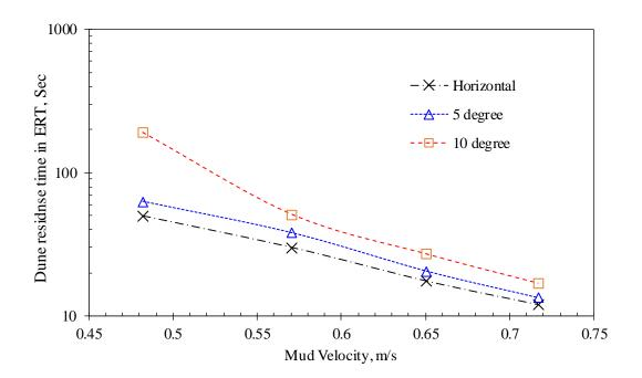
Figure 5-21: Dune moving time recorded by ERT system for fluid LV.
