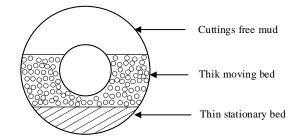
Thick moving layer, thin stationary bed: Three-layer model
