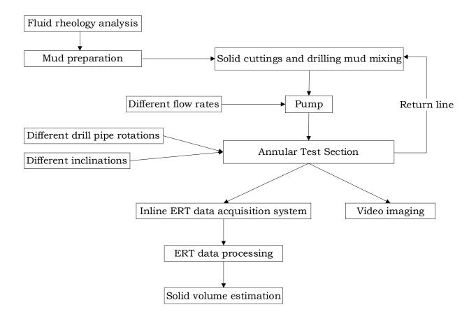
Figure 6-6: Simplified experimental procedure flowchart.
