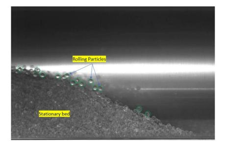
Figure 3-19: Rolling particles and stationary bed.
