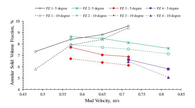
Figure 6-9 : Effect of inclination and fluid rheology on annular solid volume fraction
