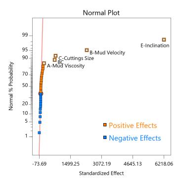
Figure 6-35: Half normal plot for pressure drop.
