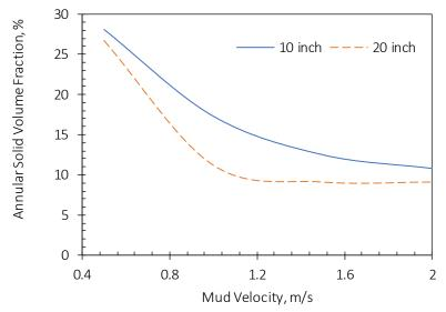
Figure A.13: Contour impact of radius of curvature in the bend section on cuttings transport.
