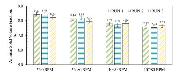
Figure 5-22: Repeatability test for different operating conditions with fluid MV at 0.7 m/s
