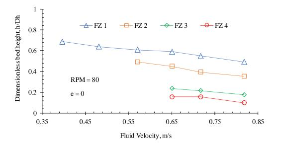
Figure 4-17: Variations of bed thickness for different fluid rheologies and mud velocities.4.3.4 Moving Bed Velocity Estimation
