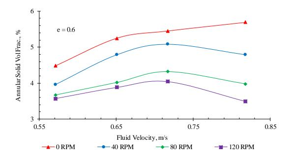
**Figure 3-15**: Annular volume fraction for highly eccentric annulus (e = 0.6)
