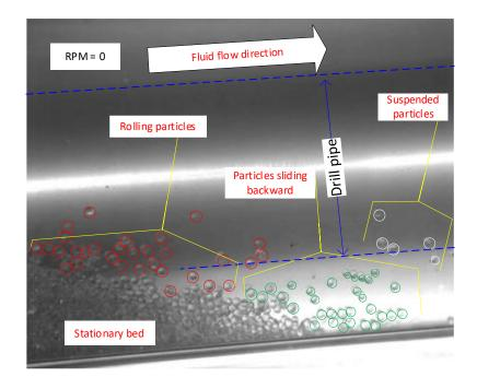
**Figure 5-15**: High-speed camera visualization of solid particles movement (RPM = 0)
