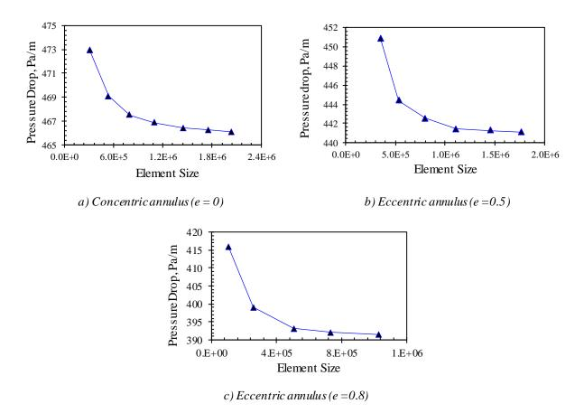
Figure 2-3: Grid independence study for all three annular configurations.
