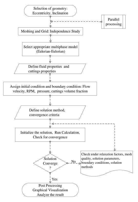
Figure 2-4: Flow chart of CFD simulation.
