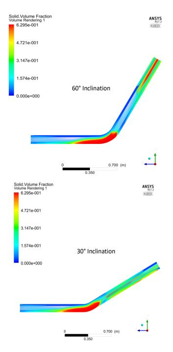
Figure A.8: Contour map of solid accumulation in inclined bend.
