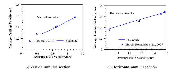
Figure 2-6: Cuttings velocity as a function of fluid velocity
