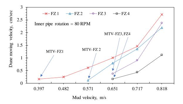
Figure 4-15: Minimum transport velocity (MTV) for different fluids
