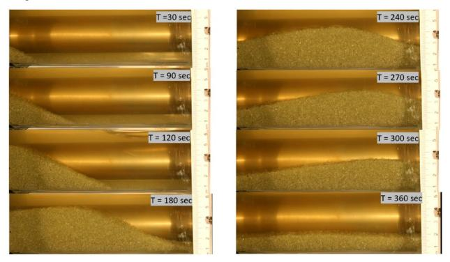
Figure B.1: Transient dune movement pattern at mud velocity 0.482 m/s with FZ 1.
