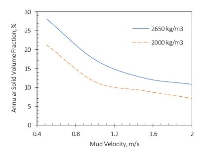
Figure A.11: Effect of cuttings density on hole cleaning.
