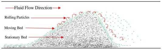
Figure 4-8: Front view of schematic of dune movement in a horizontal section
