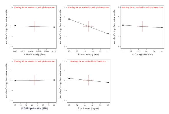
Figure 6-32: Mean dependency of annular concentration on other parameters
