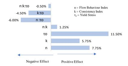
Figure 2-8: Main effects and parameter interactions of drilling mud on CTE
