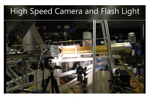
Figure B.8: Lab Image of high-speed camera and flashlight during an experiment.
