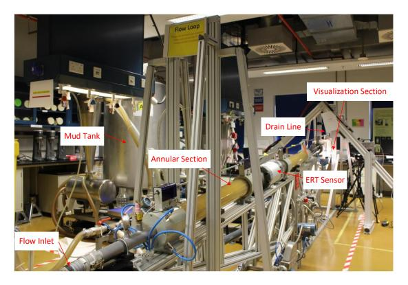
Figure 6-5: Experimental set up image at 5° inclination
