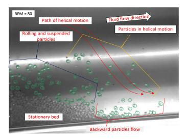
Figure 5-17: Inclined well with inner pipe rotation.
