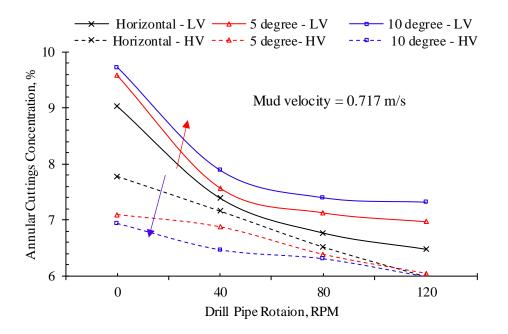
Figure 5-24: Effect of inclination on fluid rheology
