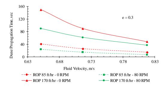
Figure 3-18: Effect of rate of penetration (ROP) on dune propagation time (e = 0.3)
