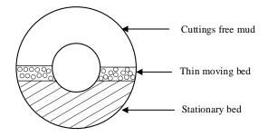
Thin moving layer, thick stationary bed: Three-layer model
