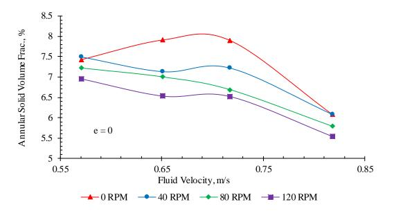
**Figure 3-14**: Annular volume fraction for concentric annulus (e = 0)
