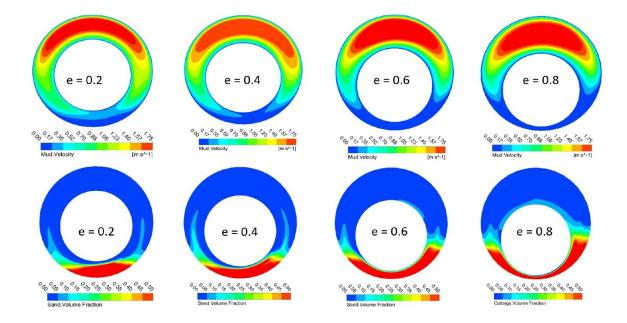
Figure 2-19: Mud velocity contour and cuttings volume fraction for different eccentricities.
