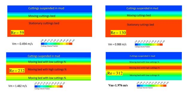
Figure 2-14: Stationary cuttings bed movement with increasing the mud velocity.
