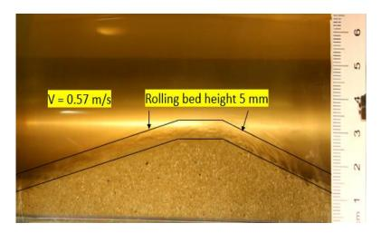
Figure 3-5: Low rolling bed height at low fluid velocity
