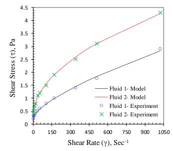
Figure A.2: Fluid rheology estimation from shear stress vs. shear rate curve.
