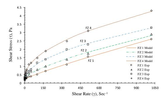
Figure 6-8: Shear stress vs. shear rate behavior for fluids FZ 1, FZ 2, FZ 3 and FZ 4
