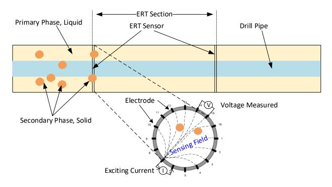
Figure 5-6: Schematic of ERT sensor
