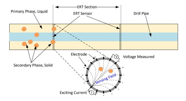
Figure 6-7: Schematic of ERT sensor (Huque et al., 2021b)
