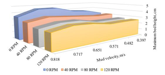
**Figure 4-16**: Maximum solid bed height for different mud velocities and drill pipe rotation *Effect of fluid rheology on bed thickness.* **Figure 4-17** shows the variation of dimensionless bed thickness with fluid FZ 1, FZ 2, FZ 3 and FZ 4 at an inner pipe rotation of 80 RPM and different
