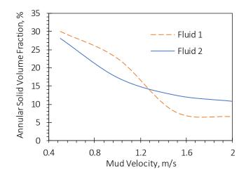
Figure A.6: Effect of fluid rheology on solid transport in bend section.
