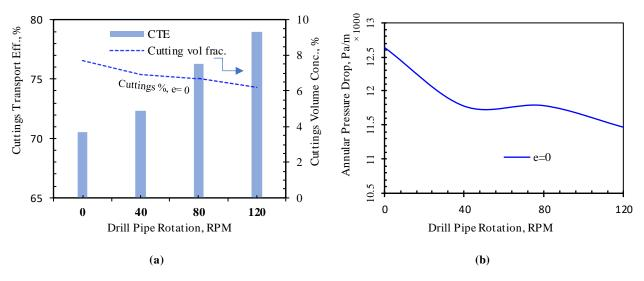
Figure 2-12: Effect of drill pipe rotation on CTE
