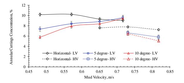
Figure 5-23: Effect of mud velocity at different inclination angles
