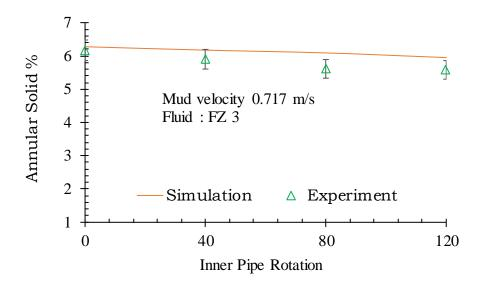
Figure 6-11: CFD model validation. Experimental data vs. Simulation result
