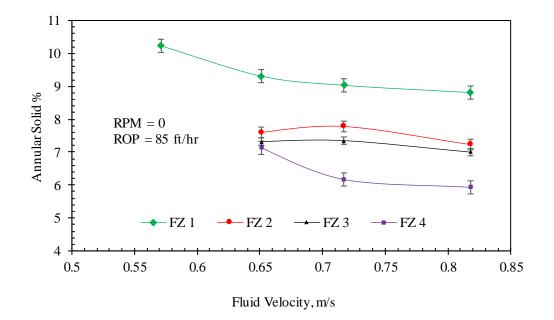
**Figure 4-14**: Annular solid volume fraction for four different fluids based on ERT data. Increasing fluid viscosity decreases the solid volume in the sand dune ( $\mu_{FZ1} < \mu_{FZ2} < \mu_{FZ3} < \mu_{FZ4}$ ).
