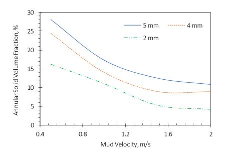
**Figure A.10:** Effect of cuttings size on hole cleaning. [Smaller cuttings are easier to clean from the bend.]
