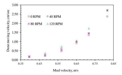
**Figure 4-18**: Solid dune velocity versus fluid velocity at different drill pipe rotations (4 % solid with FZ 1)
