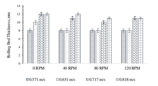
Figure 3-7: Rolling bed height variation with fluid velocities and drill pipe rotations (e = 0)
