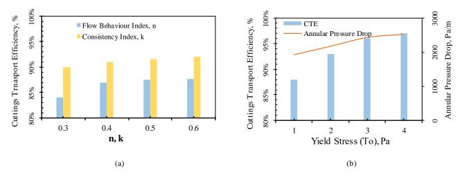
Figure 2-10: Cuttings transport efficiency as a function of a) n and k; b) yield stress (to)
