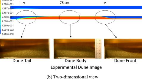
Figure 6-13: Solid dune movement along the annular section
