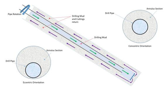
Figure 2-1: Cuttings transport in the annular section with concentric and eccentric profile.
