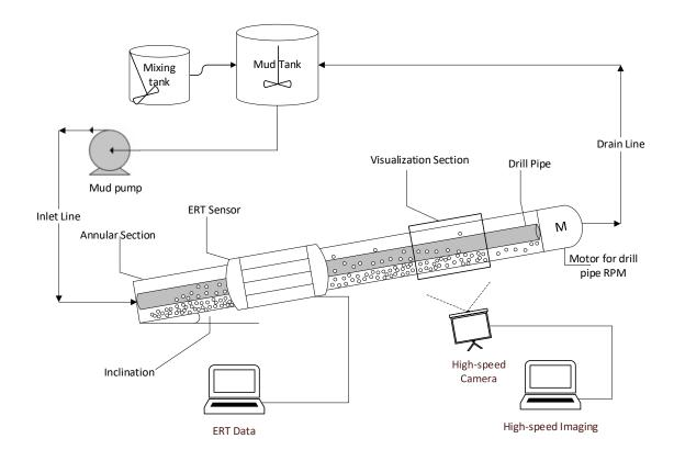
Figure 6-4: Experimental section schematic
