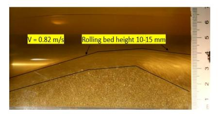
Figure 3-6: High rolling bed height at high fluid velocity
