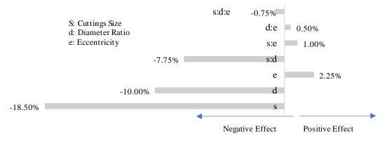
Figure 2-15: Main effects and interactions of cuttings size, annular clearance, eccentricity.
