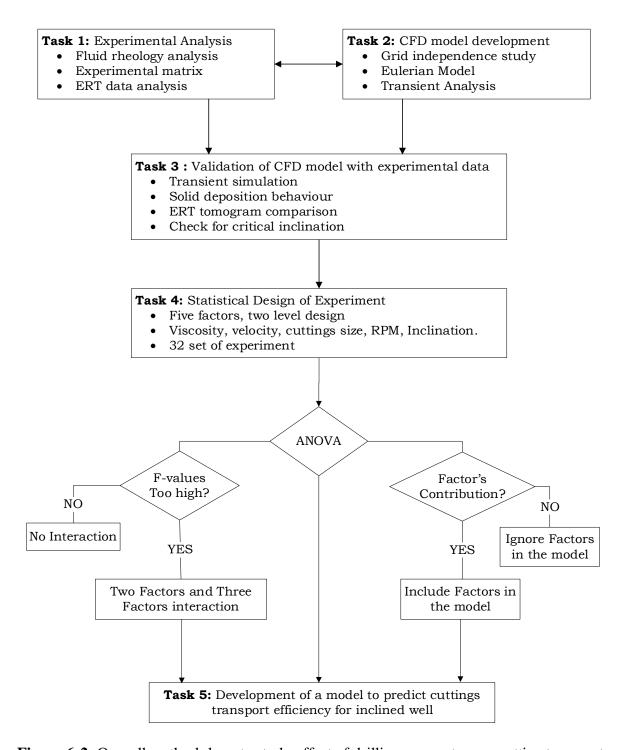
**Figure 6-2:** Overall methodology to study effect of drilling parameters on cutting transport. Task 4 focuses on five factors - two level design of experiment (DOE) and ANOVA. Task 5 includes the statistical CTE model development and validation using artificial neural network (ANN).
