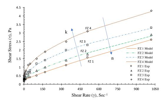
Figure 4-6: Shear stress vs. shear rate behavior for fluids FZ 1, FZ 2, FZ 3 and FZ 4
