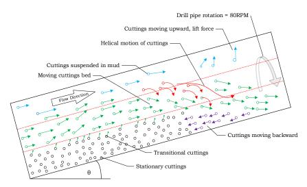
Figure 5-18: Schematic of cuttings transport in inclined well with inner pipe rotation
