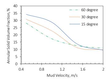
**Figure A.7:** Effect of inclination on solid transport in bend section. [At higher mud flow rate, inclination effect in negligible.]
