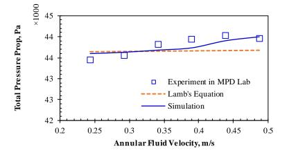
Figure 2-7: Total pressure drop comparison with managed pressure drilling experiment.
