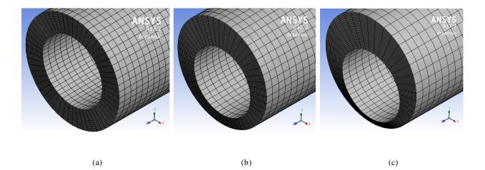
Figure 2-2: Computational mesh for different annular configurations
