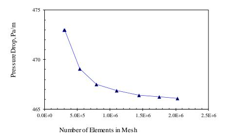
Figure 6-3: Grid study for concentric annular section
