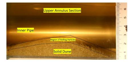
Figure 3-3: Visualization section showing solid dune, annulus section, and inner pipe.
