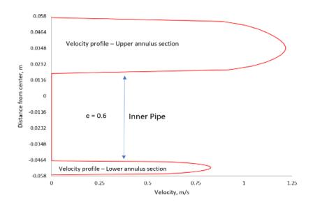
Figure 3-10: Annular velocity profile for a highly eccentric annulus
