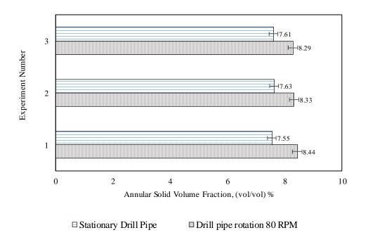
**Figure 4-7**: Repeatability test results for a slurry pump rate of 270 LPM (≈ 71 GPM)
