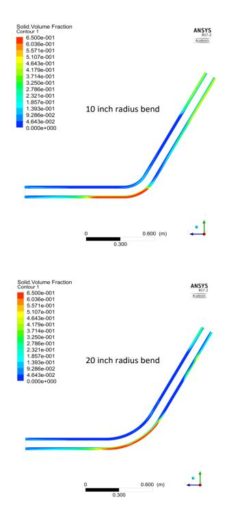
Figure A.14: Contour of cuttings accumulation on 10 in. Curvature and 20 in. Curvature.
