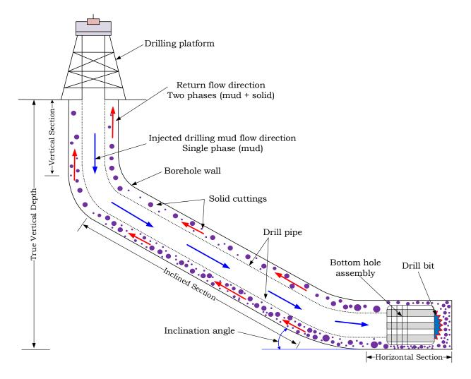
Figure 6-1: Schematic of cuttings transport in inclined drilling operation
