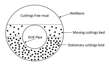
Figure 4-9: A cross-sectional view of three-layer model of cuttings transport
