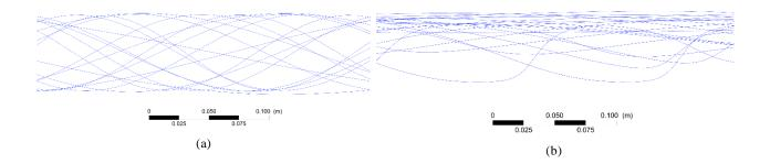
Figure 2-18: Mud velocity streamlines in a) a concentric annulus; b) an eccentric annulus.
