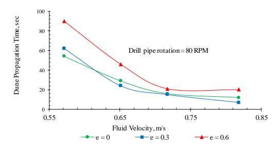
Figure 3-13: Sand dune propagation time for drill pipe rotation of 80 rpm
