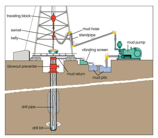
Figure 1-1: Rotary drilling and mud circulation system (Encyclopaedia Britannica, 2017)
