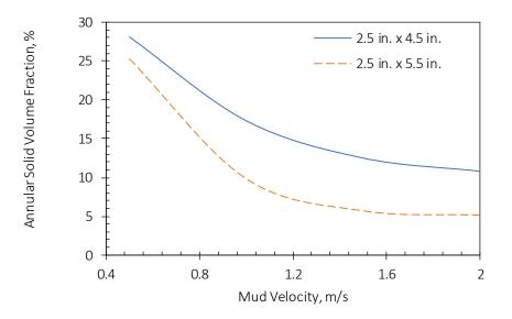
Figure A.12: Effect of annular clearance on hole cleaning.
