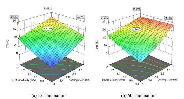
Figure 6-20: Effect of inclination on cutting transport efficiency.
