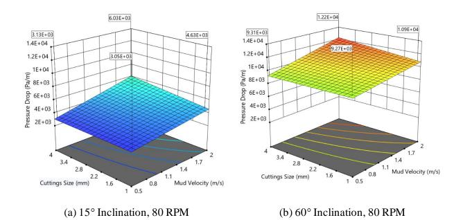
Figure 6-37: Velocity-Cuttings size interaction on pressure drop.
