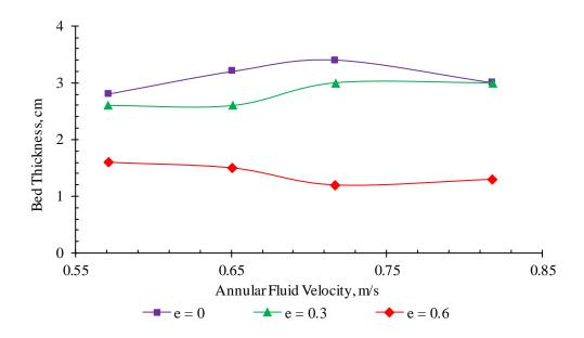
Figure 3-9: Effect of eccentricity on annular bed height at 40 RPM
