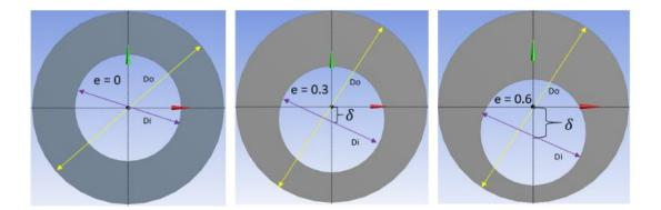
Figure 3-8: Different eccentric annular position used in this study.
