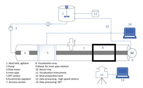
Figure 4-2: TAMUQ multiphase flow loop experimental schematic
