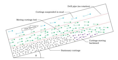
Figure 5-16: Cuttings moving in inclined well with no inner pipe rotation.
