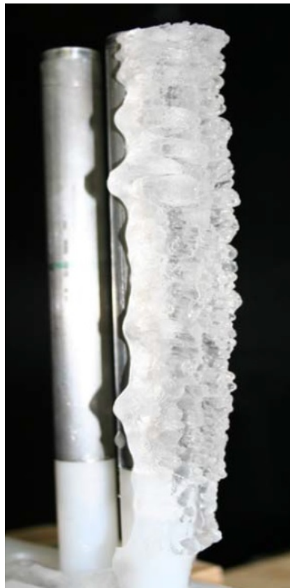
Figure 1.9: Ice detection method using cylindrical probes
