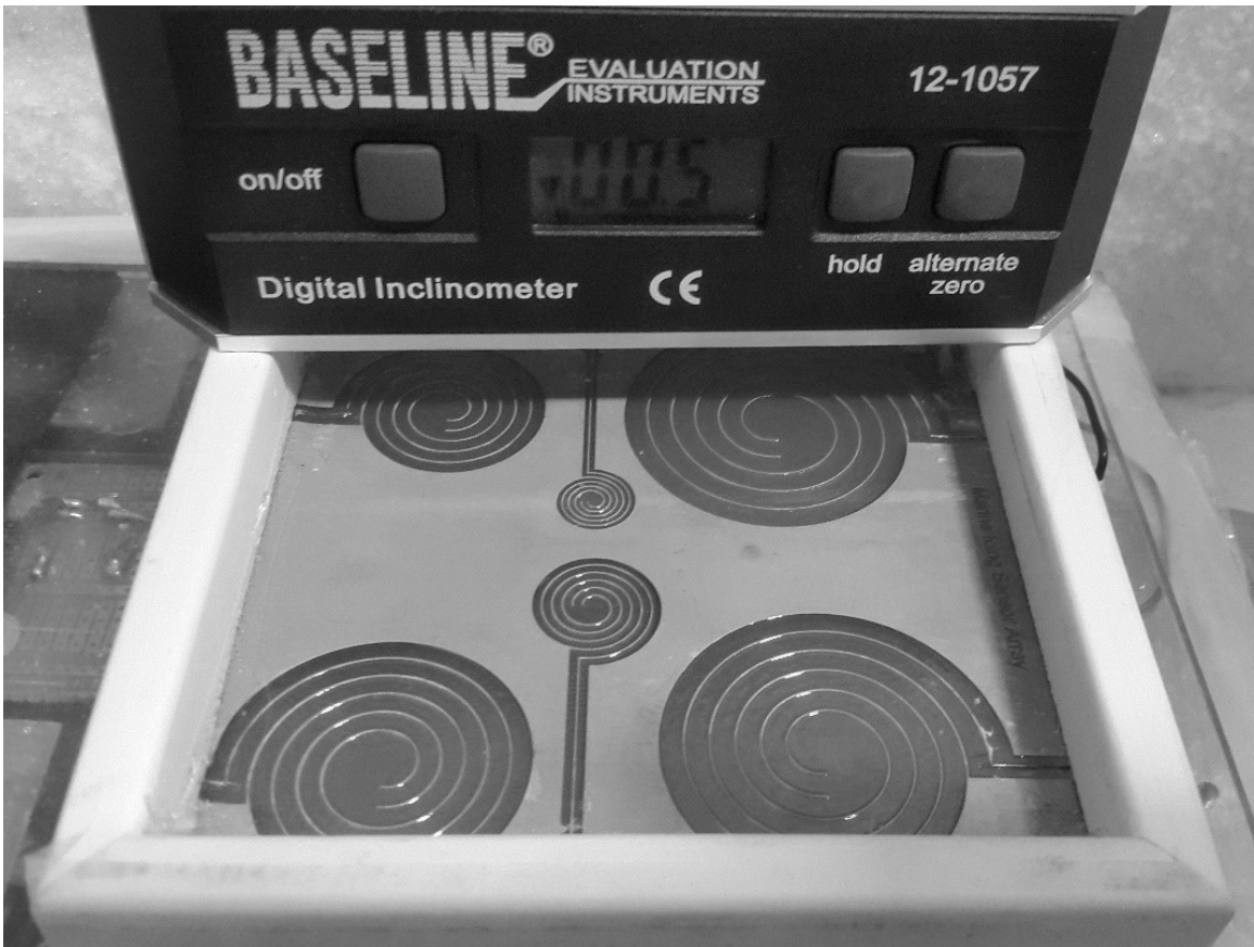
Figure 3.7: Sensor Leveling prior to the Experiment
