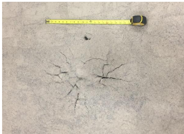
Figure 3.10: Soil failure mode observed (Test D-1)
