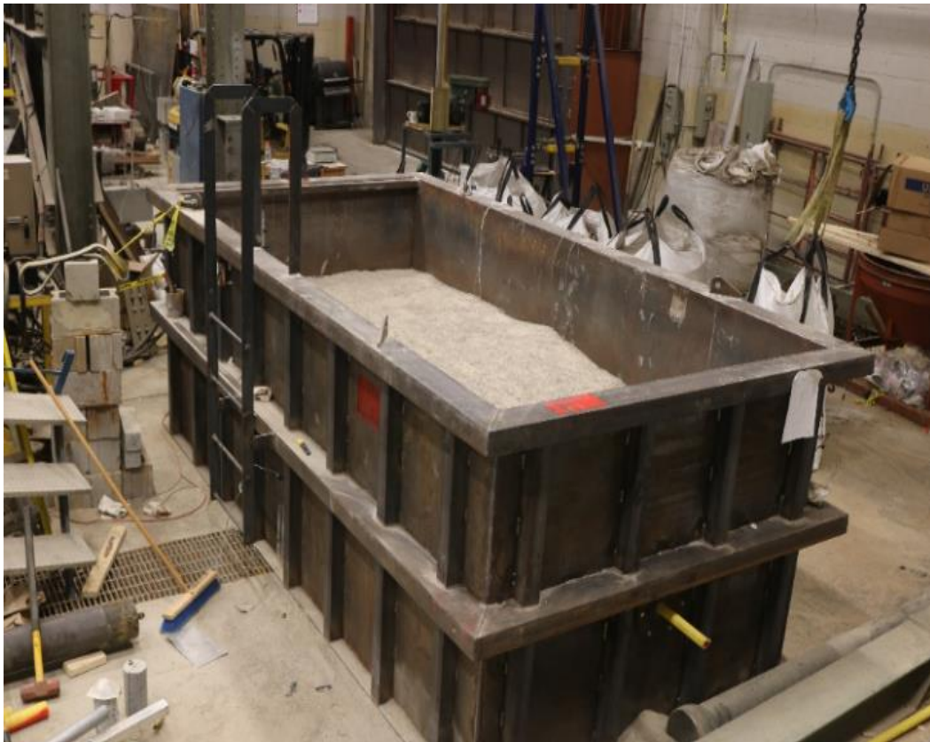
Figure 3.4: Test facility for soil-pipe interaction testing
