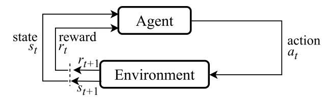
Figure 3.4: Diagram showing the flow in RL of state and reward information from the environment to the agent, and actions from agent to environment.
