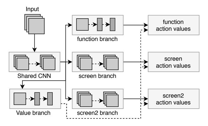
Figure 4.2: Diagram showing overall design of the network.
