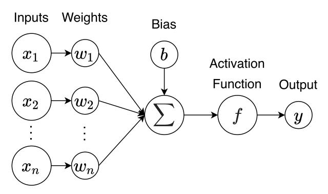
Figure 3.2: Diagram showing the calculation of an artificial neuron's output:  $y = f(b + \sum x_i w_i)$ .
