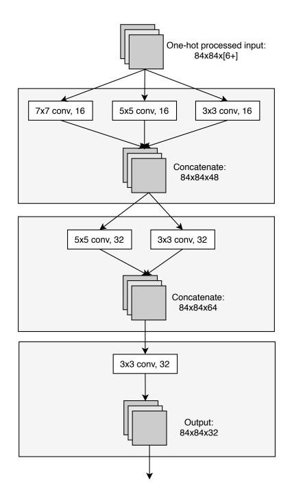
Figure 4.3: Diagram showing the shared CNN. The processed input has a different number of layers (6 or more) depending on the input features used. Convolutional filters all have stride 1, and are described as "[filter dimensions] conv, [# filters]".
