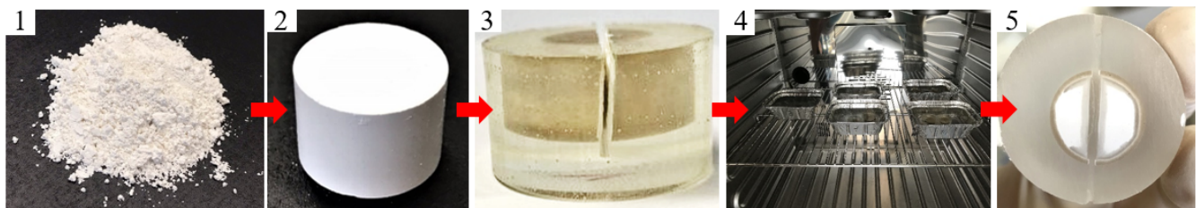
Figure 3.25. Schematic procedure of Ca(OH) 2 carbonation experiments.
