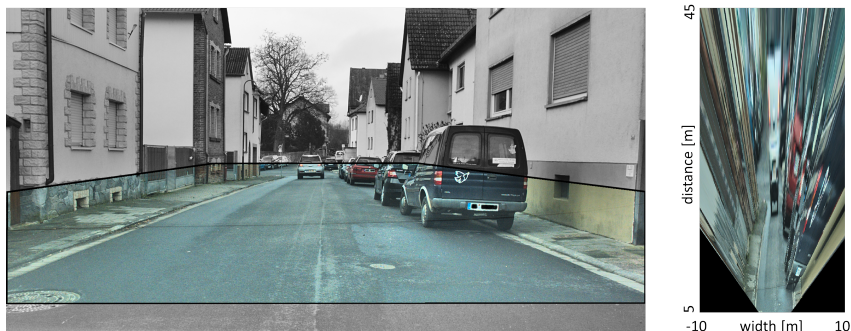
Figure 4.3: Example street scene image of the BMAG domain. The patches that are extracted from the image in perspective view (left) are limited to the corridor highlighted by colored pixels. The corridor is determined by a limitation of the metric Bird’s-Eye-View area (right).
