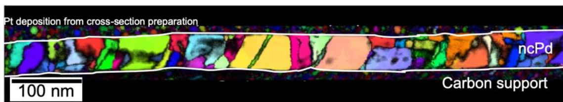
Figure 3-9 Orientation map of a cross-section of nc palladium thin film deposited on carbon substrate showing the projection effects (modified from [206]).
