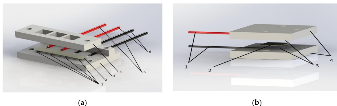
Figure 1. Schematic images of cells used in impedance spectroscopy studies for in-plane and through-plane geometries of the polymer film. In-plane geometry (a): 1, platinum contacts (5, current; 6, potential); 2, membrane; 3, bottom Teflon plate; 4, upper Teflon plate. Through-plane geometry (b): 1, platinum contacts; 2, membrane; 3, platinum foil; 4, upper and bottom Teflon plates.
