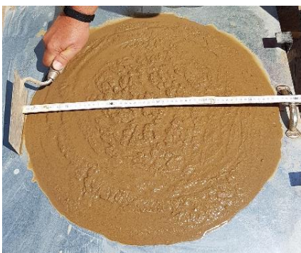
Figure 12: TFB Consistency test on site
