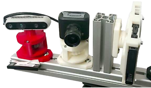
Figure 2: Physical setup used in the experiments (Sect. 4.1). From left to right: Intel RealSense, Prophesee Gen3S1.1 event camera and Sony Mobile point projector MPCL1A. Our method is designed for the point projector and the event camera, here separated by a 11 cm baseline. The Intel RealSense D435 sensor is only used for comparison.
