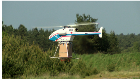
Fig. 1: Unmanned DLR superARTIS research helicopter with drop system for humanitarian needs.
