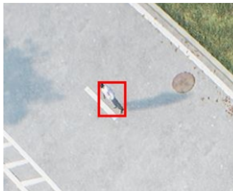
Fig. 4: Generated image of a human by AIRSIM labeled by a bounding box.
