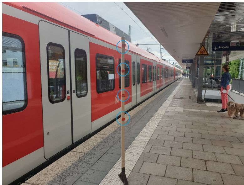
Figure 2: Rigid wooden structure containing four magnetometers at 1.7 m, 1.4 m, 1.1 m and 0.8 m. The magnetometers have been highlighted in the figure with blue circles.
