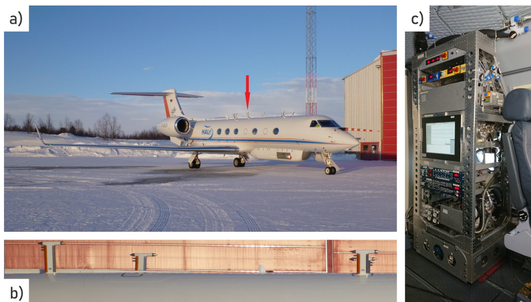
Figure 3.1.: (a) The HALO research aircraft during the POLSTRACC campaign. The red arrow marks the inlet position for AIMS. (b) Detail of the top of the fuselage with four trace gas inlets. (c) The AIMS instrument inside the cabin. Tubing at the ceiling connects the inlets to the instrument.
