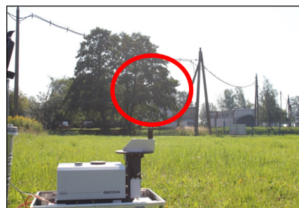
Figure 4.7: EM27/SUN measurement location roughly 50 m downwind of a coal mine ventilation shaft (red circle).
