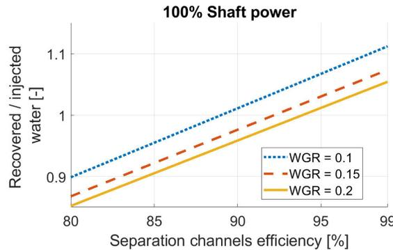
**Fig. 13 Effects of separation channels efficiency for different WGR.**
