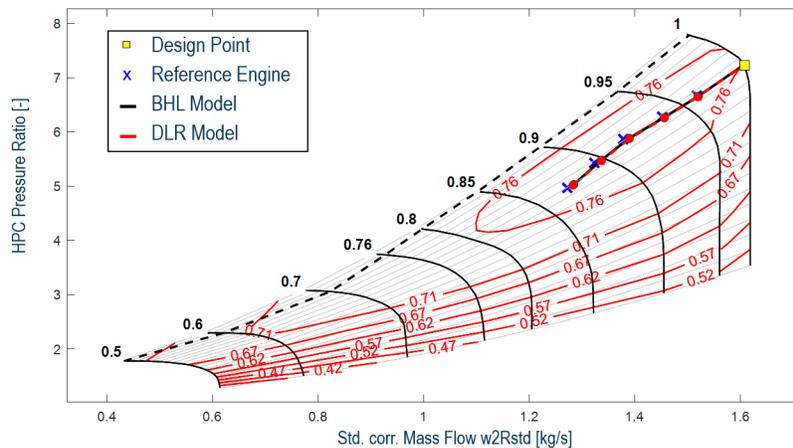
**Fig. 5 Operating line on compressor map with modeled data points and reference values.**
