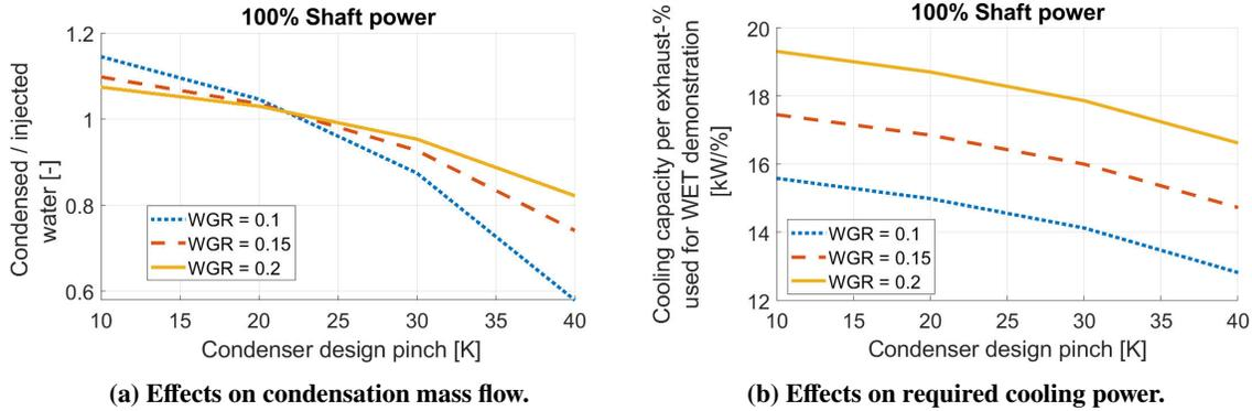
**Fig. 12 Condenser design pinch variations for different water to gas ratio (WGR).**
