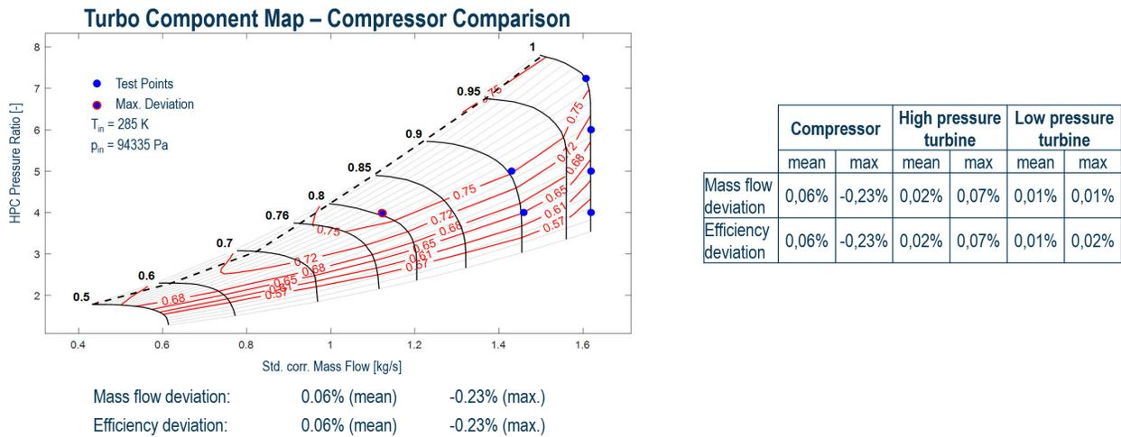
**Fig. 4 Turbomaps comparison between DLR and BHL.**
