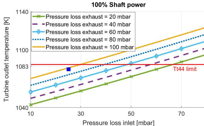
**Fig. 10 Impact of pressure losses on  $T_{t44}$  at full load.**
