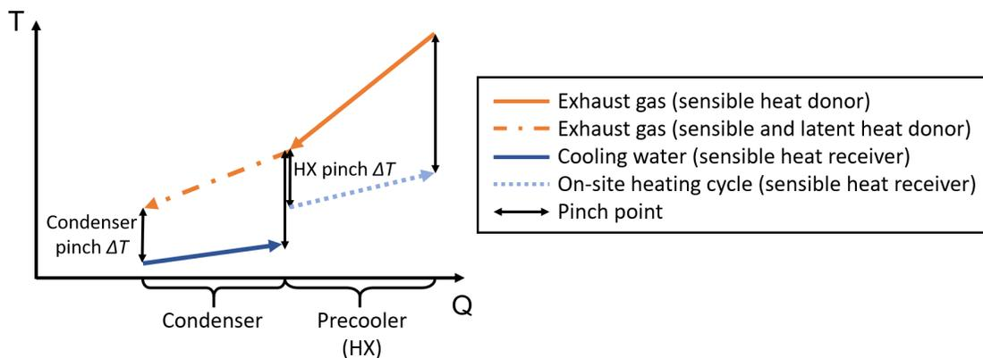
**Fig. 6 Pinch points diagram for the heat exchanger and for the condenser.**
