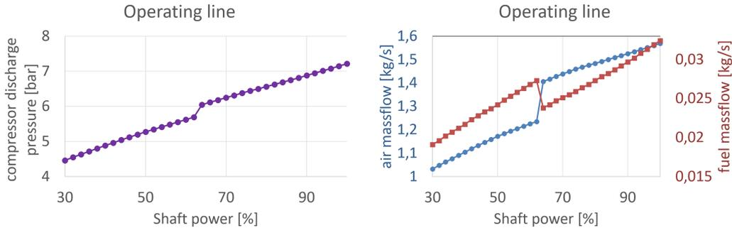
(a) Effects on compressor discharge pressure. (b) Effects on air and fuel flow entering the burner.
