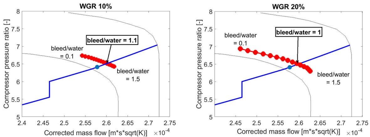
**Fig. 11** Variation of additional bleed flow on the compressor map for the WET-M250 test rig at full load.
