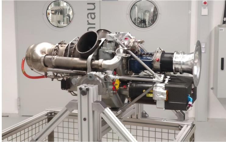
**Fig. 2 M250-based GenSet in the DLR laboratory.**
