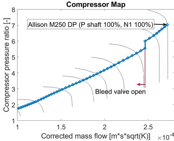
Fig. 7 Effects of opening/closing of the bleed valve on the compressor operating line.
