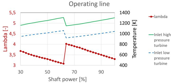
**Fig. 9 Behavior of lambda and turbines inlet temperatures.**
