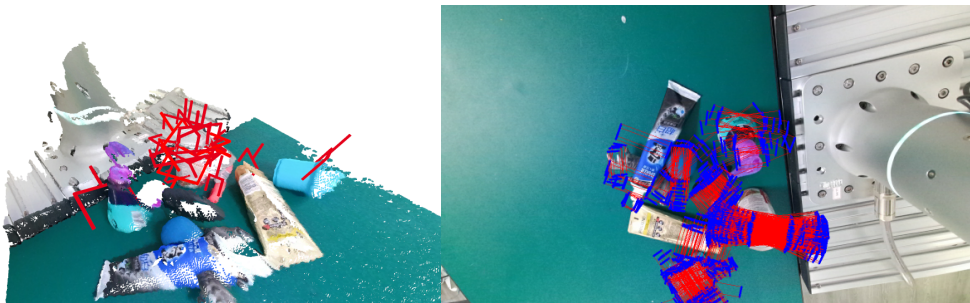
Figure 2.2: 6-DoF (left panel) to 2D planar (right panel) grasp conversion using GraspNet-1Billion dataset’s ground truth grasps.
