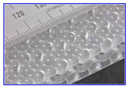
Fig. 12: Additive manufactured suction panel demonstrator (Gyroid, skin porosity 1%)
