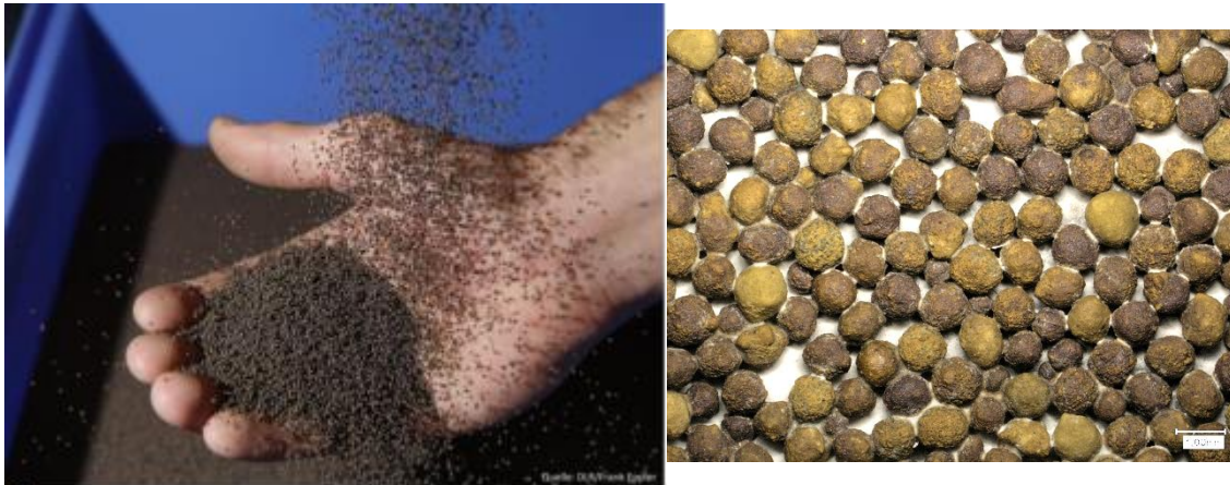
Bauxite based "proppants" produced for fracking industry
