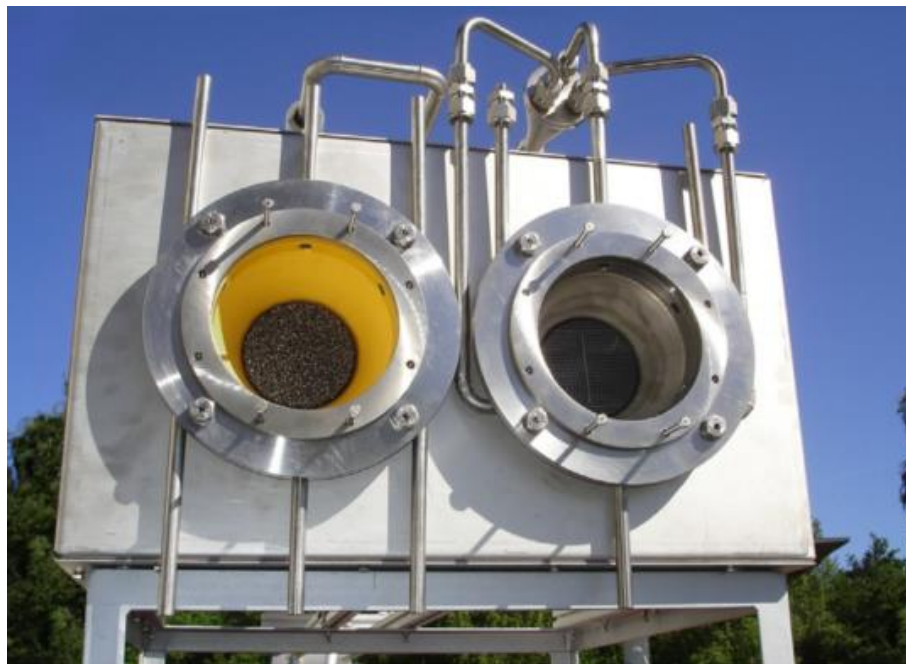
Figure 2-6: actual two-chamber solar reactor with \text{H}_2\text{SO}_4 evaporator (left) and \text{SO}_3 decomposer (right) [22]
