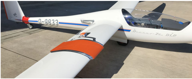
Fig. 4 The wing glove mounted on the wing of the Discus-2c for flight test
