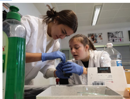
Figure 3: Producing ferro fluid out of sun flower oil and black powder for laser printers
