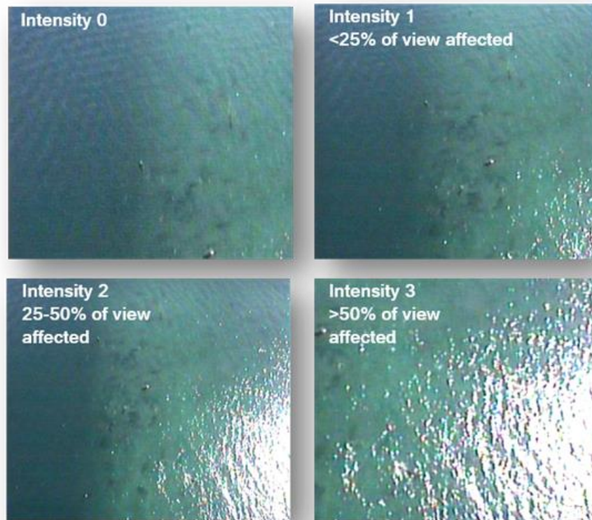
Figure 2.3. Examples of scores for the differing intensities of glare for selected UAV images obtained from Shark Bay, Western Australia. Images by Amanda Hodgson.
