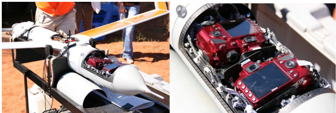
Figure 2.2. Pictures of the ScanEagle UAV (left), fitted with the two SLR cameras (right). Images by Amanda Hodgson.
