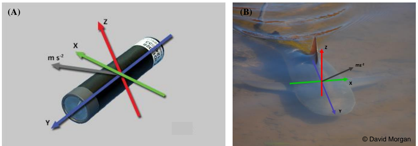
Figure 2.2: (A) Vemco V13AP coded transmitter surgically implanted into bull sharks and largemouth sawfish and (B) bull shark with arrows showing the three axes acceleration is collected from; Z (sway), X (surge) and Y (heave). Grey arrow represents VeDBA. Figure modified from Innovasea (2018).
