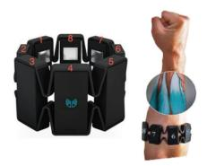
Figure 1: Myo armband and its placement on the forearm (Wahid et al., 2018)
