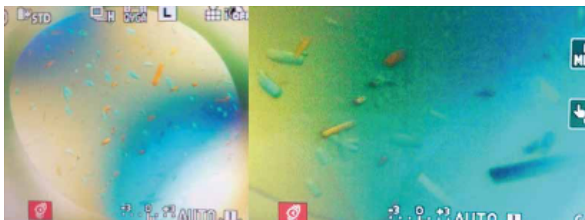
Figure 32. Bid3CCSS crystals obtained after streak seeding. To further enhance crystal growth and shape, nicely grown apo crystals from the salt screen were crushed in the crystallization buffer and subjected to a seeding protocol using a horsehair. Images show that this approach yielded non-ingrown crystals of a good size. (Images were captured using a polarization filter).
