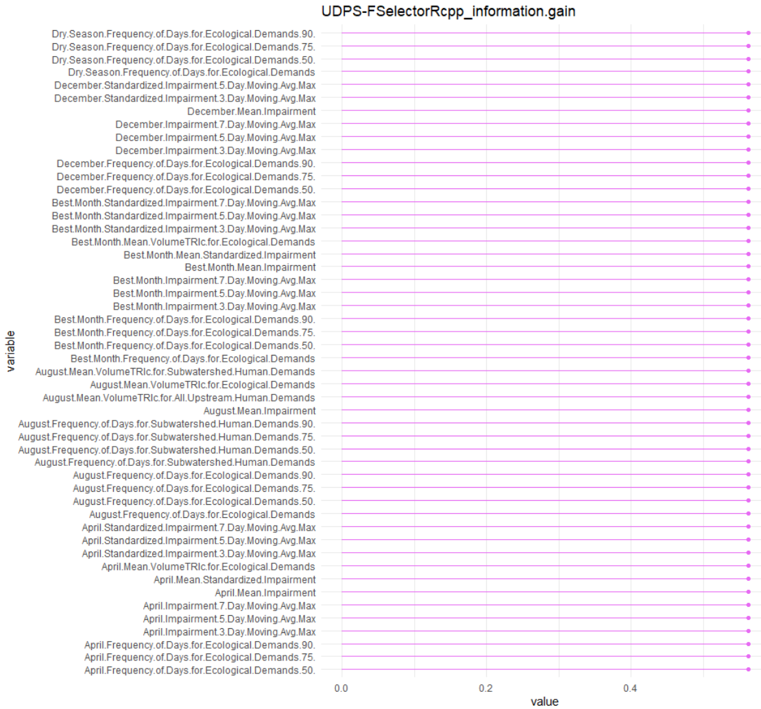
Figure 28 - Results of the feature_importance R function on UDPS using the 'FSelectorRcpp_information.gain' function, which is aimed at obtaining which predictors provide the most information gain. As can be seen, all 50 variables shown have the same result of the statistical test.
