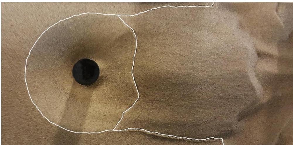
Figure 3 - Bed profile measurements for tests E1 and S1 in the XY symmetry plane at Z/D = 0 (top) and photograph of the scour formation for test S1 (bottom)
