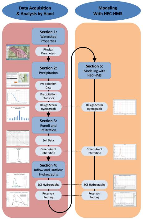
Fig. 4 Flow diagram of the sections and activities within HDC. *Note.* The sections are represented by blue rectangles and the activities are the white bubbles. Dashed lines indicate components of the modeling process that are performed both by hand or in Excel and modeled in HEC-HMS
