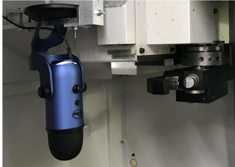
Figure 7. A microphone used in a milling operation for chatter detection.
