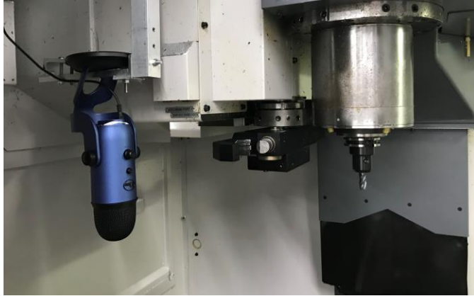
Figure 17. Experimental setup of machine tool-tool holder-end mill system and microphone.
