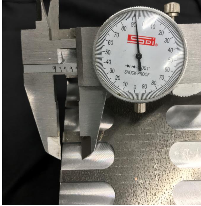
Figure 29. Caliper measurement of the chatter mark from point of tool entry into the workpiece.
