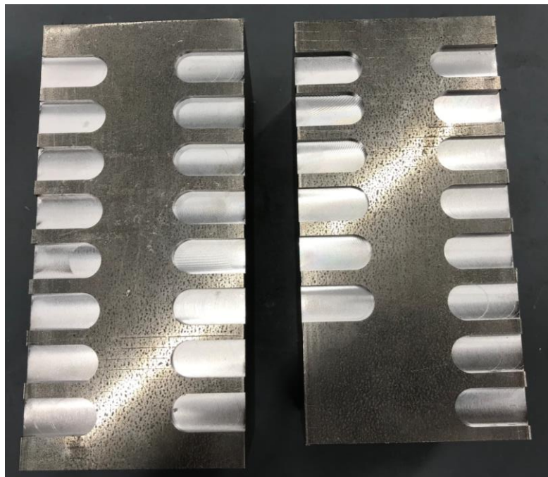
Figure 18. AISI 4140 Steel workpiece with test cuts.
