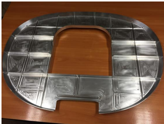
Figure 1: Aerospace component with machined thin wall ribs [21].
