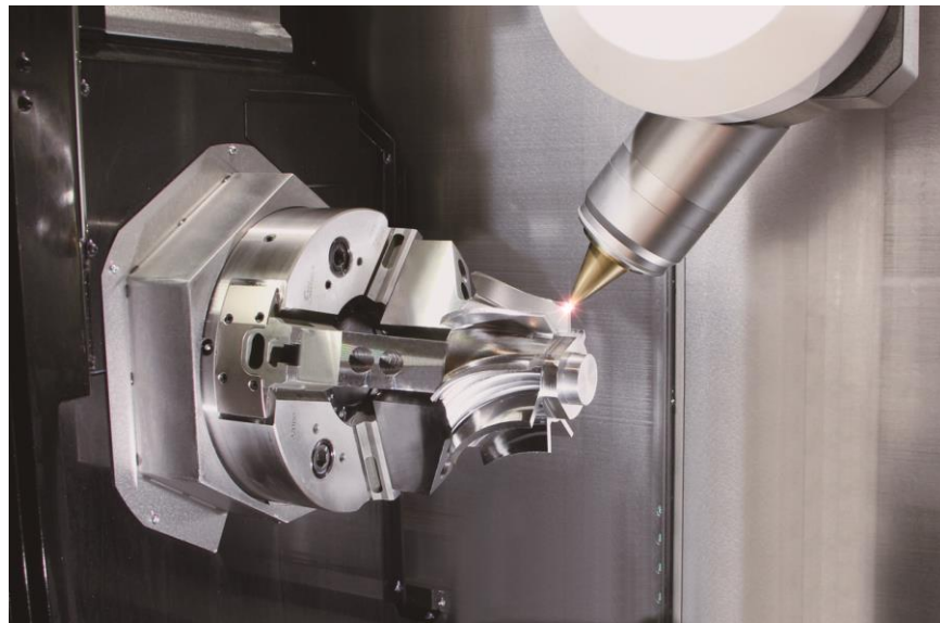
Figure 3: Mazak INTEGREX i-400AM using blown powder additive head for blade repair
