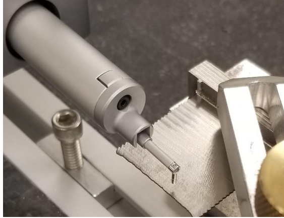
Figure 14: Contact profilometer fixturing setup
