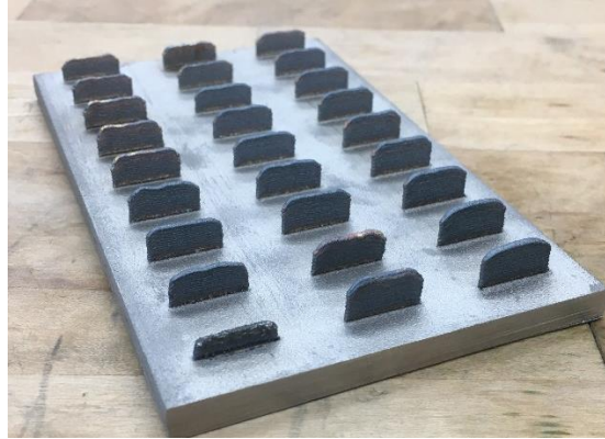
Figure 8: Parameter sweep sample for 316L powder deposition testing 27 different parameter combinations
