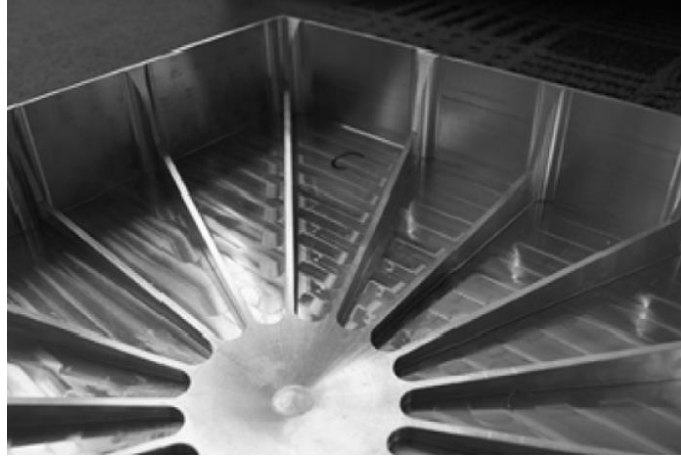
Figure 5: Thin Walled Structure using machined sacrificial supports [35].
