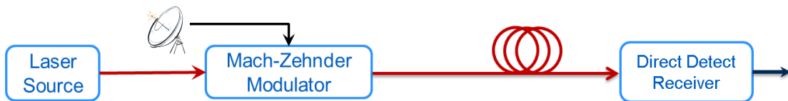
Figure 3 – Schematic of an intensity-modulated, direct detect RF photonic link.
