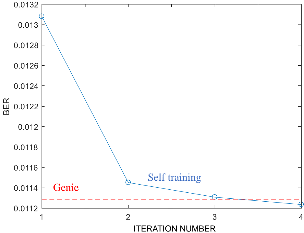
Figure 2.8: BER evolution of self-training algorithm at track pitch 26.1 nm and threshold 6.
