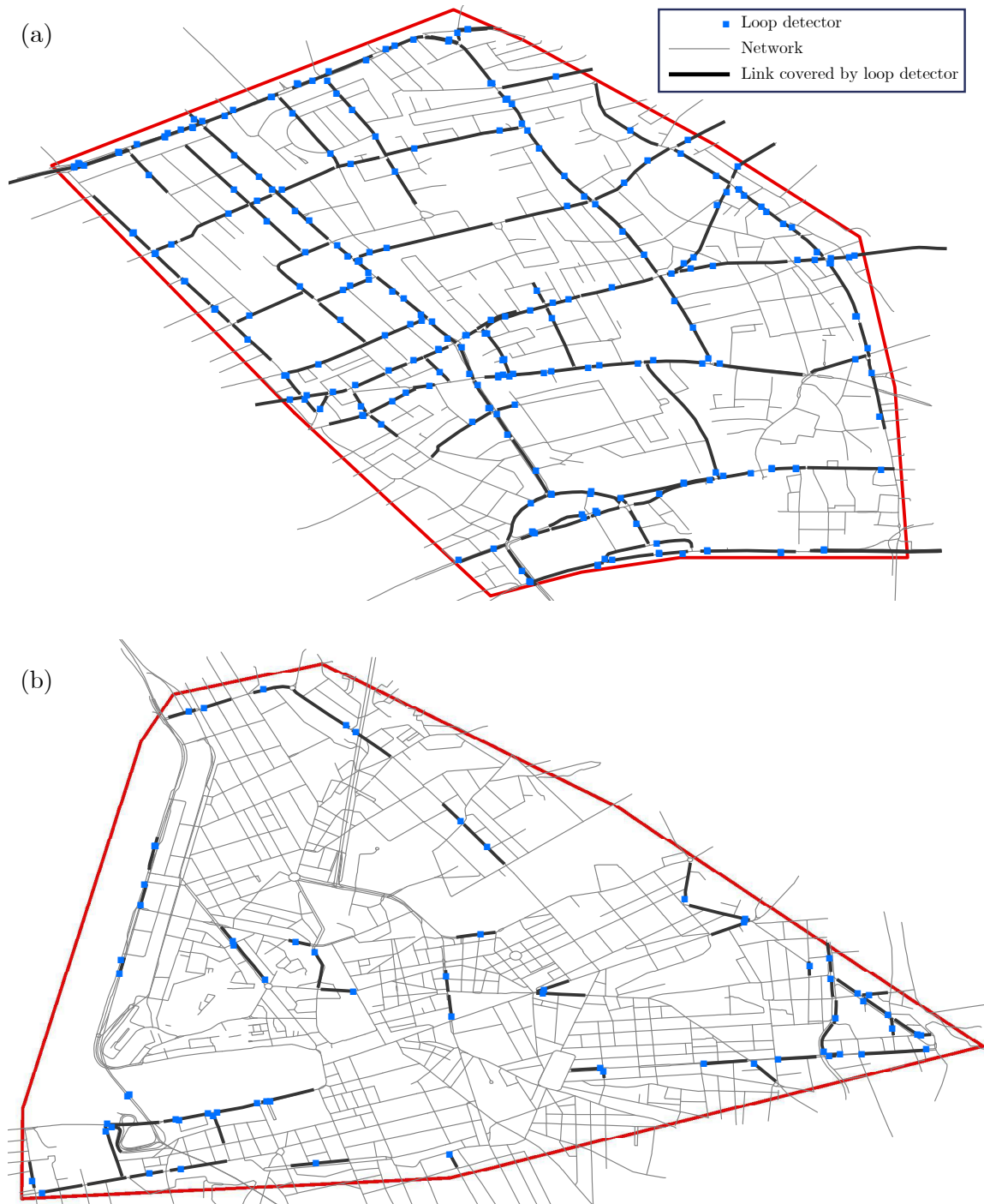
Figure 6.9: Street network and loop detectors' location and coverage for (a) London and (b) Marseille [Network maps are obtained from OpenStreetMap (2020)]
