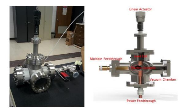
Figure 27 - Picture of the Contact Experiment Setup (left); CAD rendering of contact experiment with parts labelled (right)
