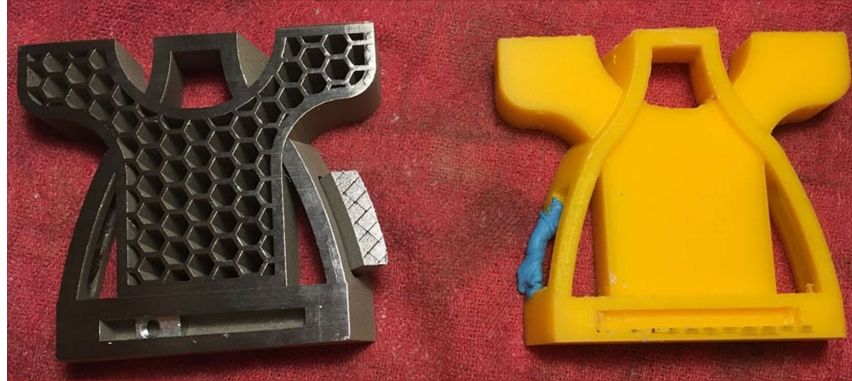
Figure 6: On the left is the printed prototype with the honeycomb pattern, as compared to a solid body prototype seen on the right.
