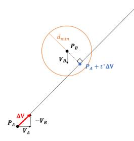
Figure A.1: Finding the distance of closest approach by reasoning geometrically in the intruder reference frame
