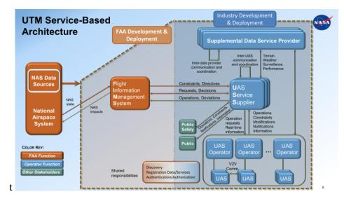
Figure 1.10: Proposed architecture for the UTM [26].
