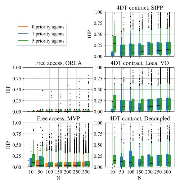
Figure 6.13: Distribution of LoS severity measured by the Horizontal Intrusion Parameter in function of agents density N for different UTM alternatives with a varying number of priority agents.
