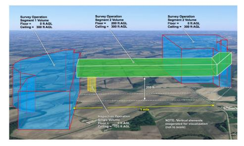
Figure 1.11: Illustration of volume reservation in the UTM (taken from FAA/NASA UAS Traffic Management Pilot Program (UPP), Industry workshop 1, March 2018).
