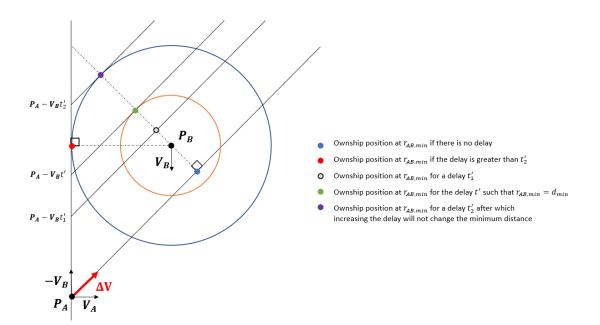
Figure A.2: Finding the distance of closest approach for different delays by reasoning geometrically in the intruder reference frame
