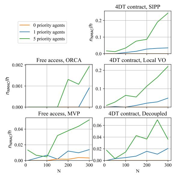
Figure 6.12: Evolution of average number of Near Mid Air Collisions per agent flight hour in function of agents density N for different UTM alternatives with a varying number of priority agents.
