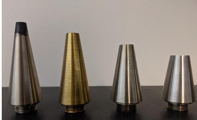
Figure 3.12 – Manufactured Centerbodies of Different Lengths
