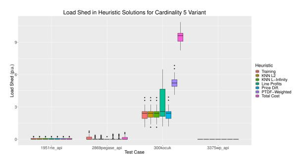
Figure 2.8: The distribution of the load shed (in per unit) for each of the heuristic solutions to the test instances which are ever infeasible.
