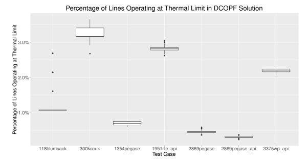
Figure C.1: Percentage of lines in each test system which have flow equal to the transmission limits when switching is not allowed for the 300 generated instances on each network.
