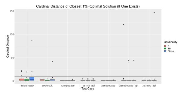
Figure 2.11: The distribution of the closest 1%-optimal solution in the training set for the 30 test instances in each test case and cardinality variant. The black horizontal line denotes a cardinal distance of 10.
