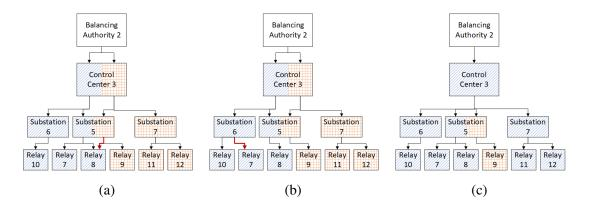
Figure 4.3: Examples of disallowed network segmentation choices. In (a), relay 8 has been assigned to both of the enclaves in substation 5, and the resulting network is no longer a forest. In (b), the original network structure is violated since relay 7 was originally a child of substation 5, but has been reassigned to substation 6. In (c), substation 5 is segmented, but both of its enclaves are assigned to the same control center enclave (see below for this restriction).
