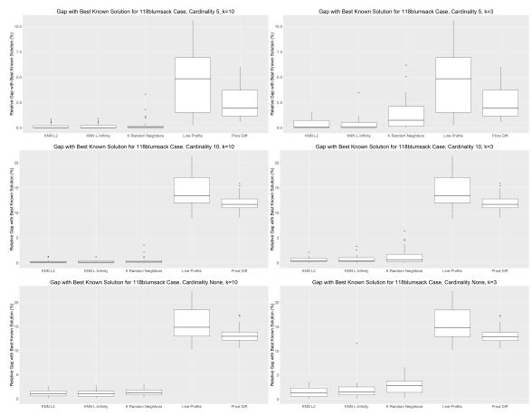
Figure 2.21: Solution quality of the k random neighbors heuristic as compared to the KNN heuristics and two of the better-performing heuristics from Ruiz, Foster, et al. (2012) on the 118blumsack case. The first column of figures uses k = 10 for the first three heuristics, and the second column uses a value of k = 3.
