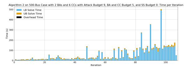
Figure 4.10: Computational time per iteration solving for a budget of 5 balancing authorities (BA) and control centers (CC), no additional substation (SS) enclaves, and an attack budget of 9 enclaves on the 500-bus case with 2 balancing authorities and 6 control centers. The color-coding scheme is the same as in Figure 4.9.
