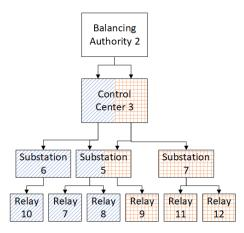
Figure 4.2: Example of a segmented portion of the control network from Figure 4.1. The balancing authority still contains one enclave, but the control center and substation 5 now contain two enclaves each. The substations and relays are patterned according to which control center enclave ultimately controls them. The enclaves in substation 5 are controlled by different parents.
