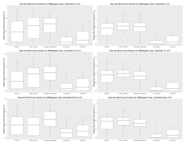
Figure 2.25: Solution quality of the k random neighbors heuristic as compared to the KNN heuristics and two of the better-performing heuristics from Ruiz, Foster, et al. (2012) on the 2869pegase case. The first column of figures uses k = 10 for the first three heuristics, and the second column uses a value of k = 3.
