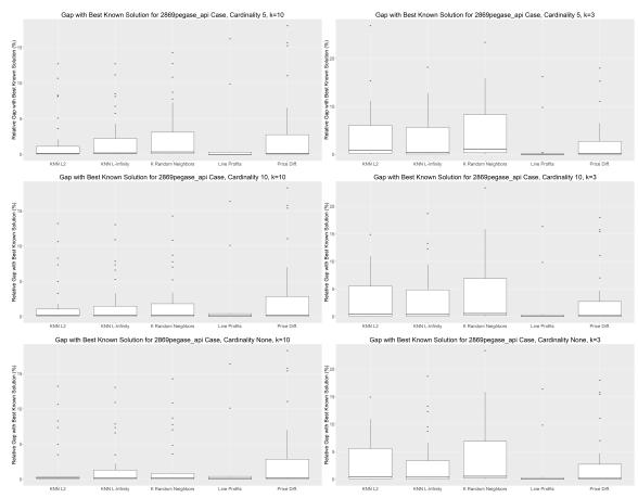
Figure 2.26: Solution quality of the k random neighbors heuristic as compared to the KNN heuristics and two of the better-performing heuristics from Ruiz, Foster, et al. (2012) on the 2869pegase\_api case. The first column of figures uses k = 10 for the first three heuristics, and the second column uses a value of k = 3.
