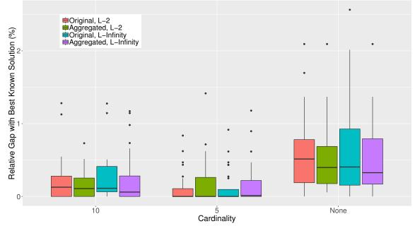
Figure 2.13: Results comparing solution quality of the KNN heuristic using the original method and using a reduced-dimension vector of net demands in each of the classes from Figure 2.12.
