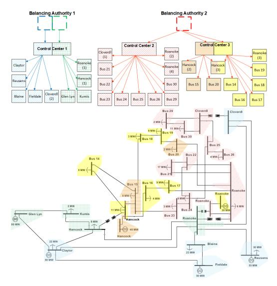
Figure 4.4: How segmentation of a 30-bus system's control network relates to the physical network. The top image displays the segmented control forest, and the lower image shows its relation to the physical grid. Each leaf node in the forest corresponds to one substation/bus on the physical grid. Substations are colored according to their parent control center enclaves.
