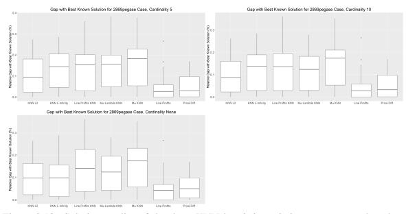
Figure 2.18: Solution quality of the three KNN heuristic variations as compared to the original KNN heuristics and two of the better-performing heuristics from Ruiz, Foster, et al. (2012) on the 2869pegase case.
