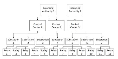
Figure 4.1: Control network structure. Balancing authorities enclaves communicate with control center enclaves which in turn communicate with substation enclaves. These then control the relays, each of which controls a set of physical grid components (i.e., lines, generators, and loads).
