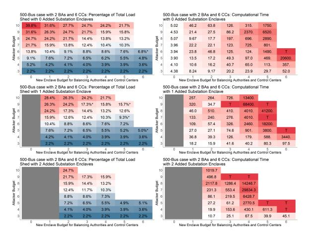
Figure 4.7: Computational results from running Algorithm 3 on the 500-bus test instance with a communication network with 2 balancing authorities (BAs) and 6 control centers (CCs).
