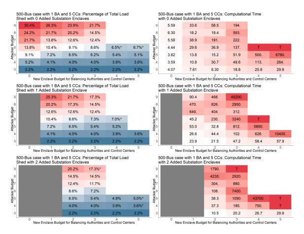
Figure 4.6: Computational results from running Algorithm 3 on the 500-bus test instance with a communication network with 1 balancing authority (BA) and 5 control centers (CCs).
