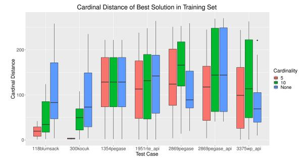
Figure 2.10: The distribution of the cardinal distances of the best solution in the training set for the 30 test instances in each test case and cardinality variant. The best solution does not tend to be close to the test instance.
