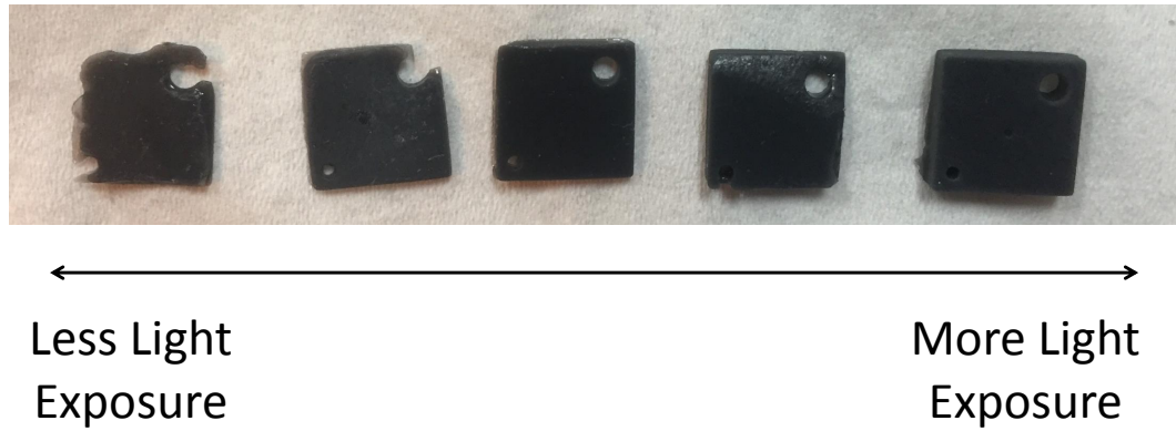
Figure 7.19: The effects of exposure time on the 3D-printed substrates.
