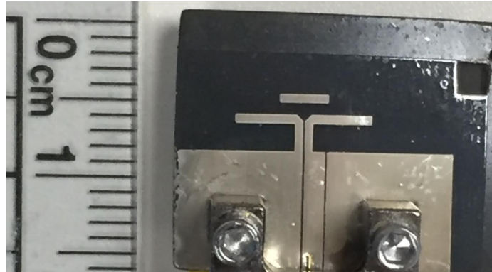
Figure 7.26: The fabricated prototype of the proposed broadband AiP design.
