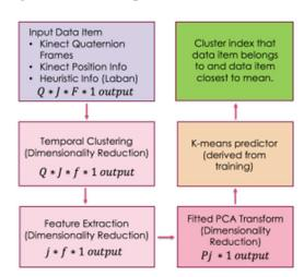
Fig. 1: Real-Time Operation
